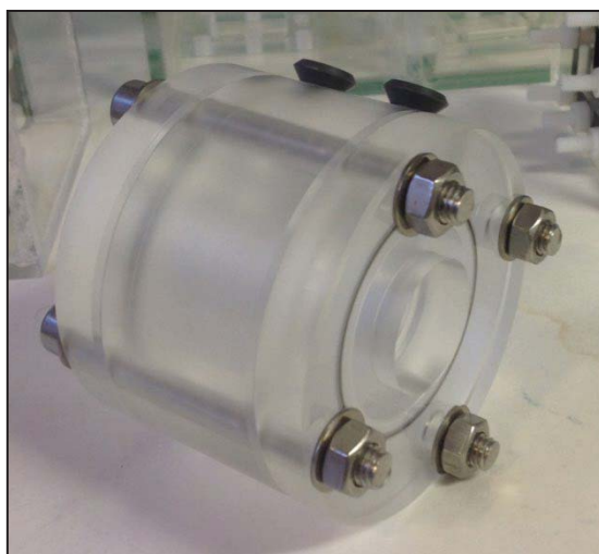
Figure 136: Photo of the constructed single chamber microbial fuel cell used in Shewanella and SRB/SOB MFC studies
