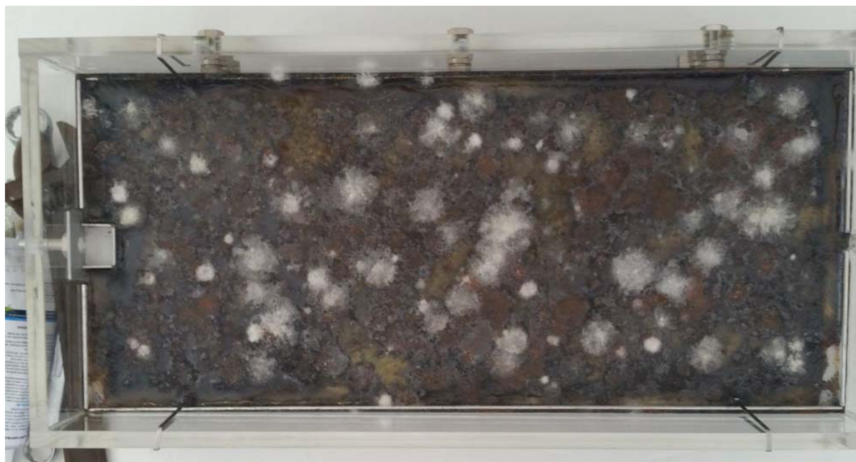
Figure 89: Top view of channel reactor showing establishment of bacterial and fungal biofilm
