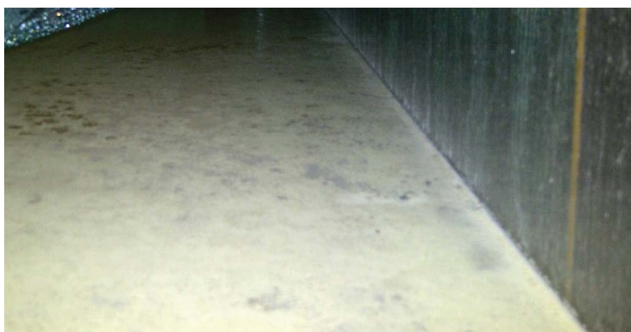
Figure 134: Photograph of the pilot scale reactor 72 hours after inoculation showing complete biofilm development.
