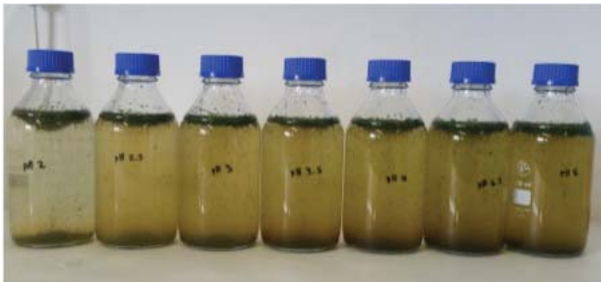
Figure 71: Photograph showing effect of initial pH on the appearance of the liquid phase (24 hours after grass addition)
