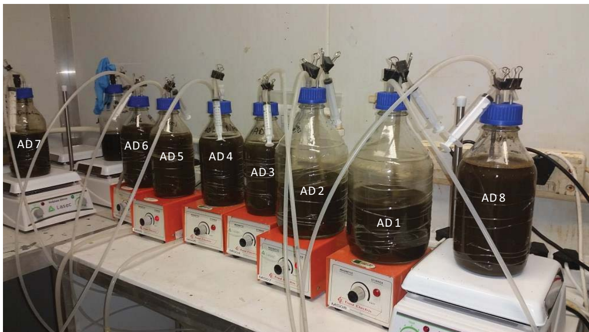
Figure 11: Experimental setup for the eight AD reactors. From left to right, Spirulina (+ve control; AD 7) reactor, Avicel reactors (AD 6 and AD 5), manure reactors (AD 4 and AD 3), grass reactors (AD 2 and AD 1) and the +ve control reactor with only inoculum (AD 8)
