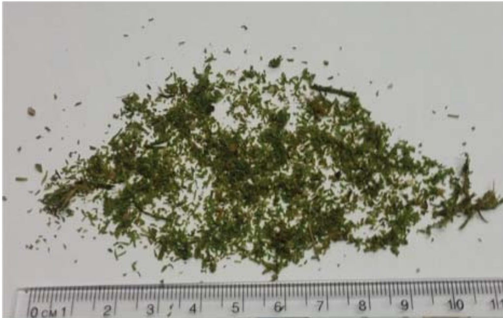
Figure 69: Photograph of the grass cuttings used, indicating the small particle size and relatively narrow size distribution.
