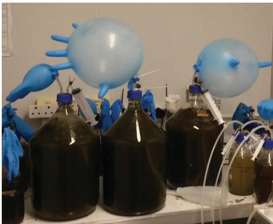
Figure 9: Stock inoculum reactor bottles (10 l) currently maintained on mixed substrates. The one 5 l inoculum reactor bottle maintained on a complex mixed algal substrate is not shown.
