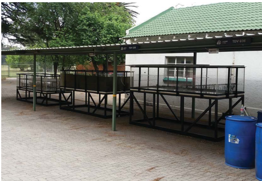
Figure 133: Photograph of the three pilot scale reactors at the pilot site. The 210 L inoculum development drums are visible in the bottom right corner
