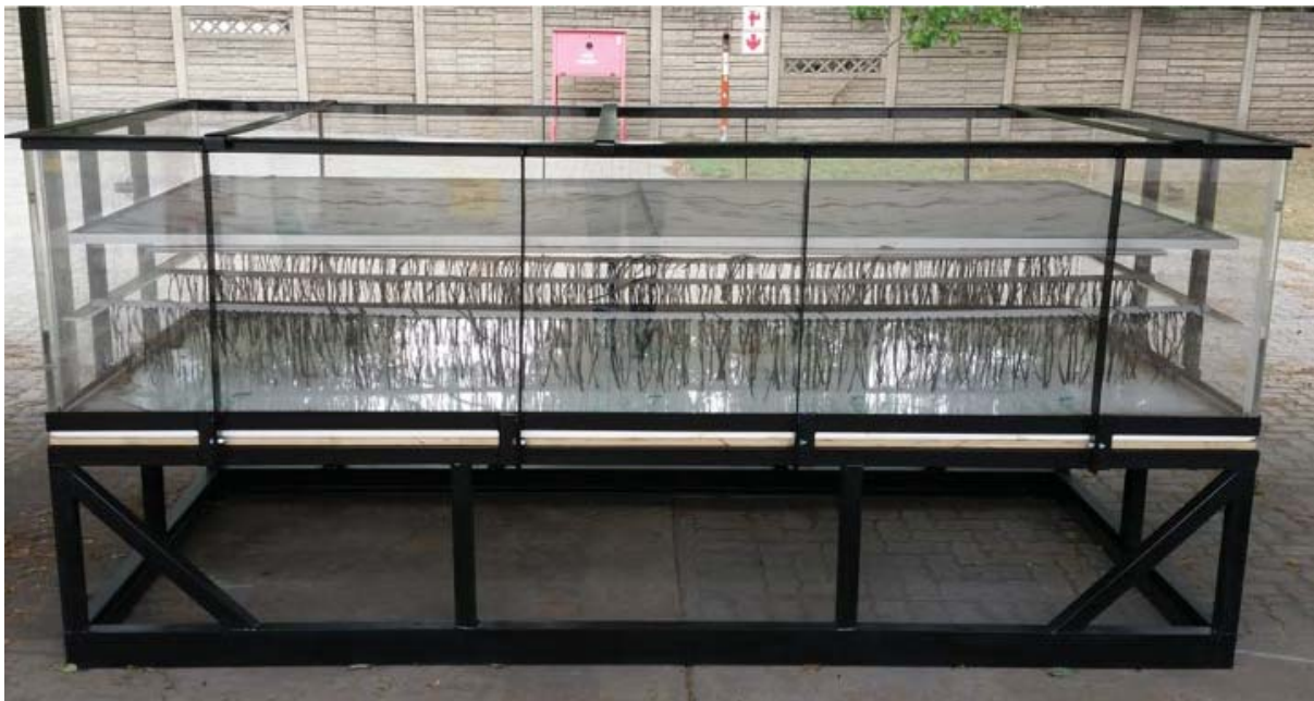
Figure 110: Image illustrating the pilot scale LFCR reactor on site, prior to inoculation
