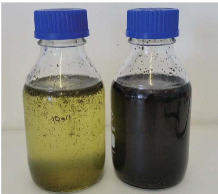
Figure 84: Evidence of sulphide generation following contact of fresh grass cuttings with raw mine water for 20 days
