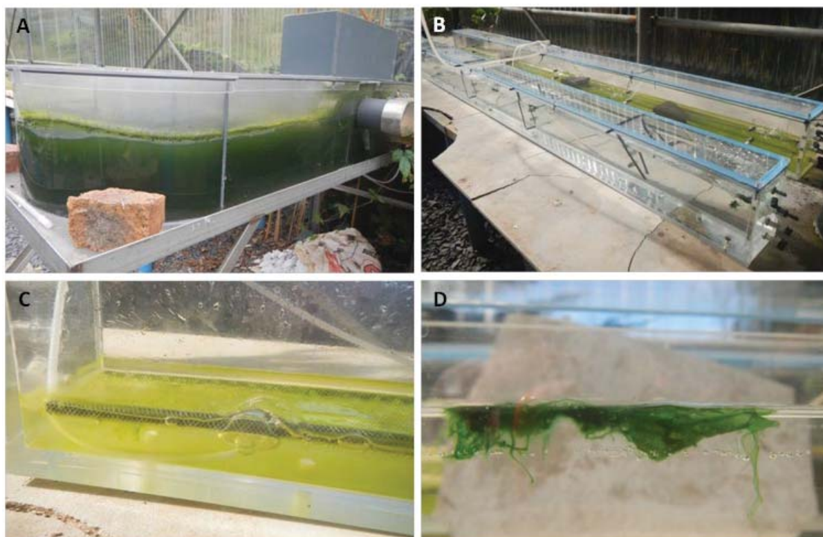
Figure 47: Larger scale reactors used for the cultivation of algal biomass. (A) Parachlorella hussii in a 70 l raceway, 25 l channel reactor for Oedogonium , (B and C) and Oscillatoria (D)
