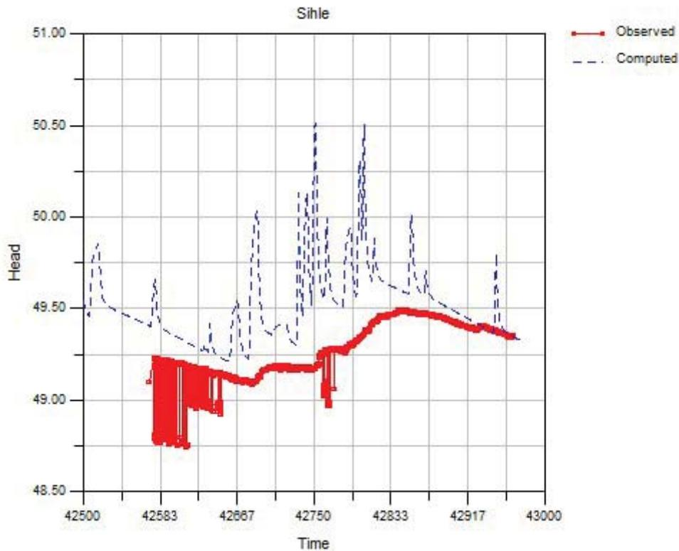
Figure 6.36 The simulated and observed heads variation for the Sihle Borehole near Vasi Pan. The large drawdown and recovery in measured head during the early monitoring period was due to short periods of abstraction.
