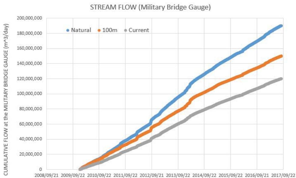
Figure 6.44 The cumulative simulated stream flow at the Military Bridge Gauge for the three different land use scenarios
