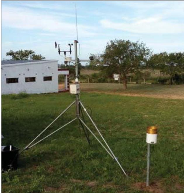
Figure 5.3 Campbell Automatic Weather Station installed at Siphesihle Bukhosini Science Centre
