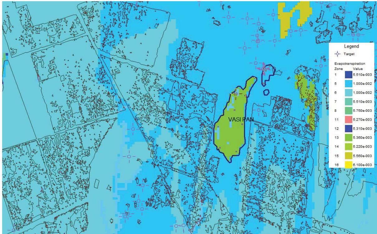
Figure 6.39 Map of the land use types used in the model to represent the Natural Conditions. The black lines show the outline of the plantations that were replaced by the natural vegetation species shown by the coloured zones. The scale shows all vegetation types, many of which are not shown in this section of the map.
