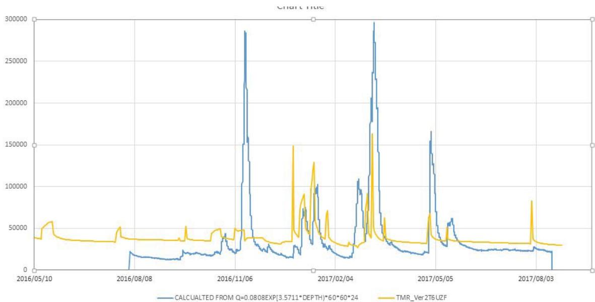
Figure 6.34 The simulated and measured transient flow rates at the Malangeni monitoring site beneath the old Military Bridge
