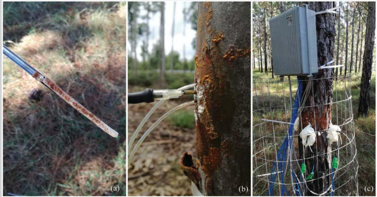
Figure 5.4 HPV installation setup at Vasi Pan, (a) assessment of sapwood depth using an incremental borer, (b) temperature thermocouples placed equidistance above and below the needle heater (c), metal fence to prevent disturbance from cattle and filler foam placed around probes to provide insulation
