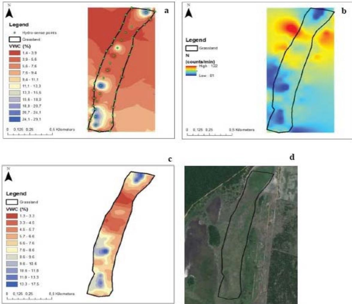
Figure 6.23 Maps of the Hydro-sense measurements (a), corrected neutron counts (b), cosmic ray rover estimates (c) and landcover (d)
