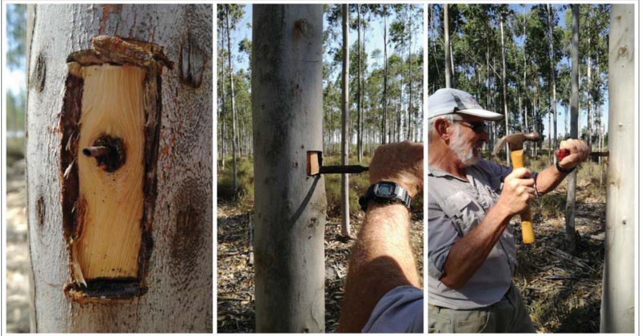
Figure 5.5 Assessment of wood density and wounding widths required for the calculation of corrected sap flow
