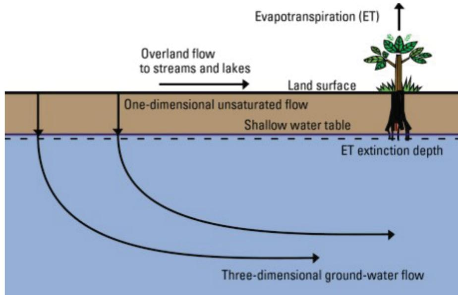
Figure 5.19 The conceptual model for the UZF package (Niswonger *et al.*, 2006)
