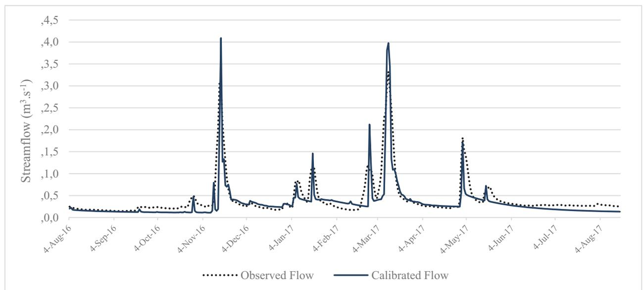
Figure 6.27 Observed streamflow (military bridge) against calibrated simulated flow
