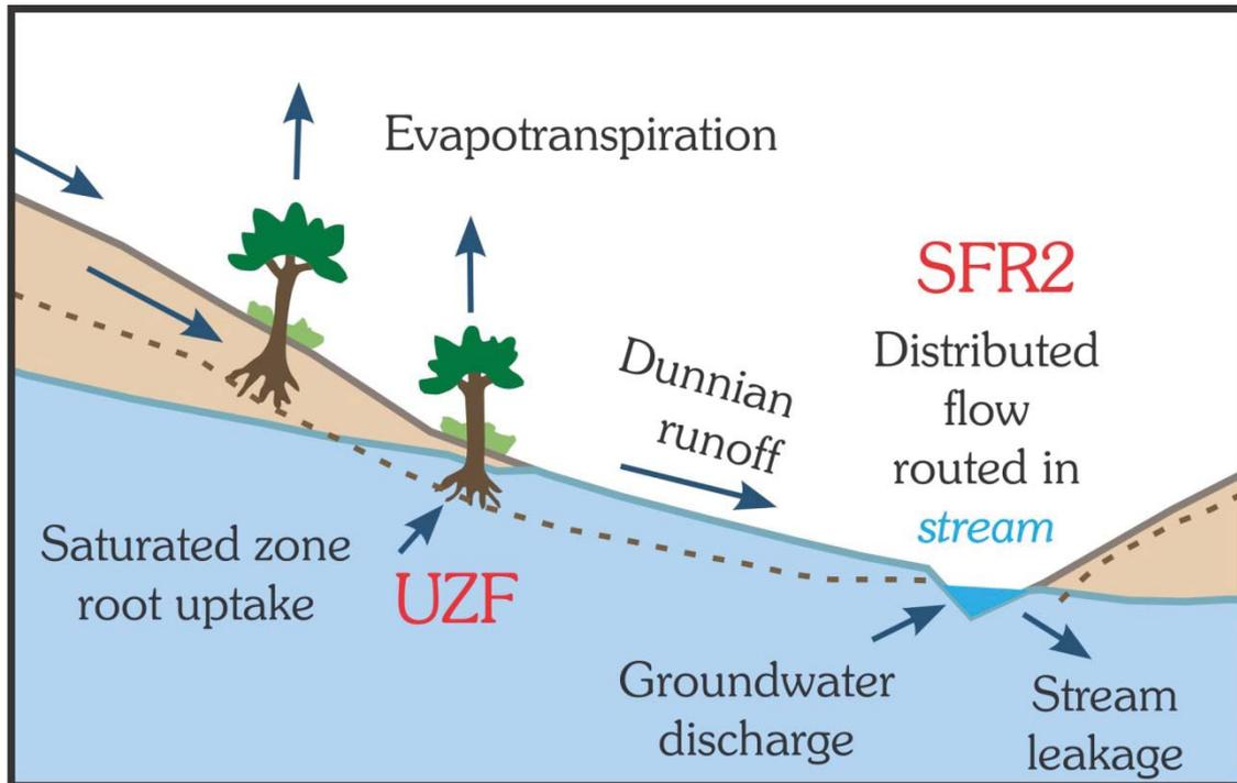
Figure 5.20 The hydrological components included in the model development for a groundwater dominated system
