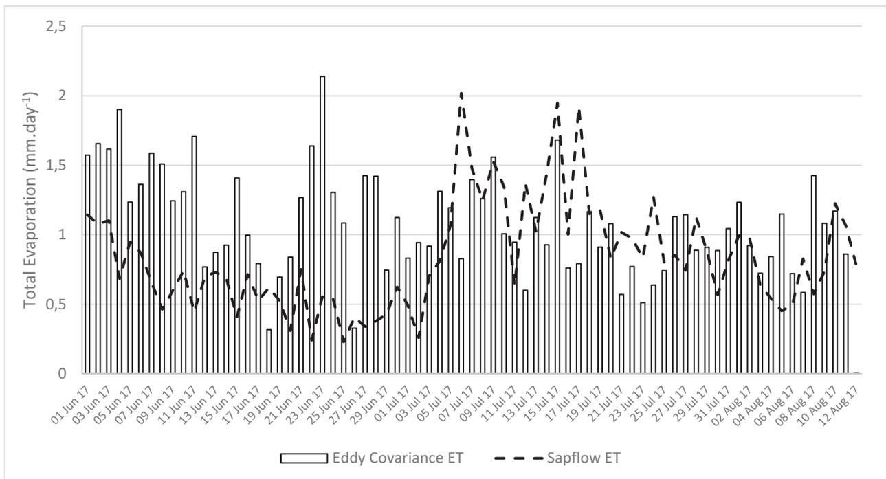
Figure 6.20 Daily total evaporation of the commercial pine stand measured using EC and sap flow techniques
