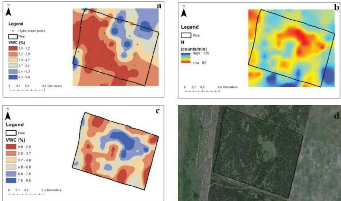
Figure 6.25 Maps of the Hydro-sense measurements (a), corrected neutron counts (b), cosmic ray rover estimates (c) and landcover (d)
