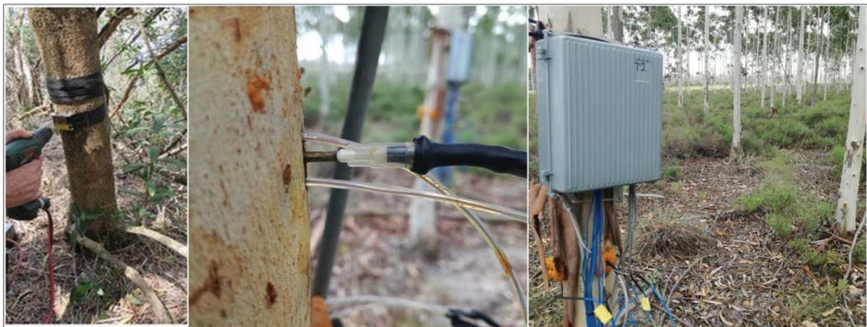
Figure 2.8 HPV equipment installed on a *Warburgia salutaris* and a *Eucalyptus grandis*, indicating the thermocouples inserted above and below a heater probe around the tree stem
