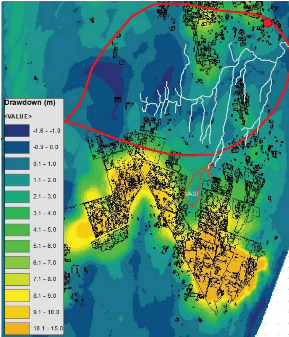
Figure 6.42 The simulated drawdown (m) in the Manzengwenya region for the current groundwater relative to the natural vegetation.
