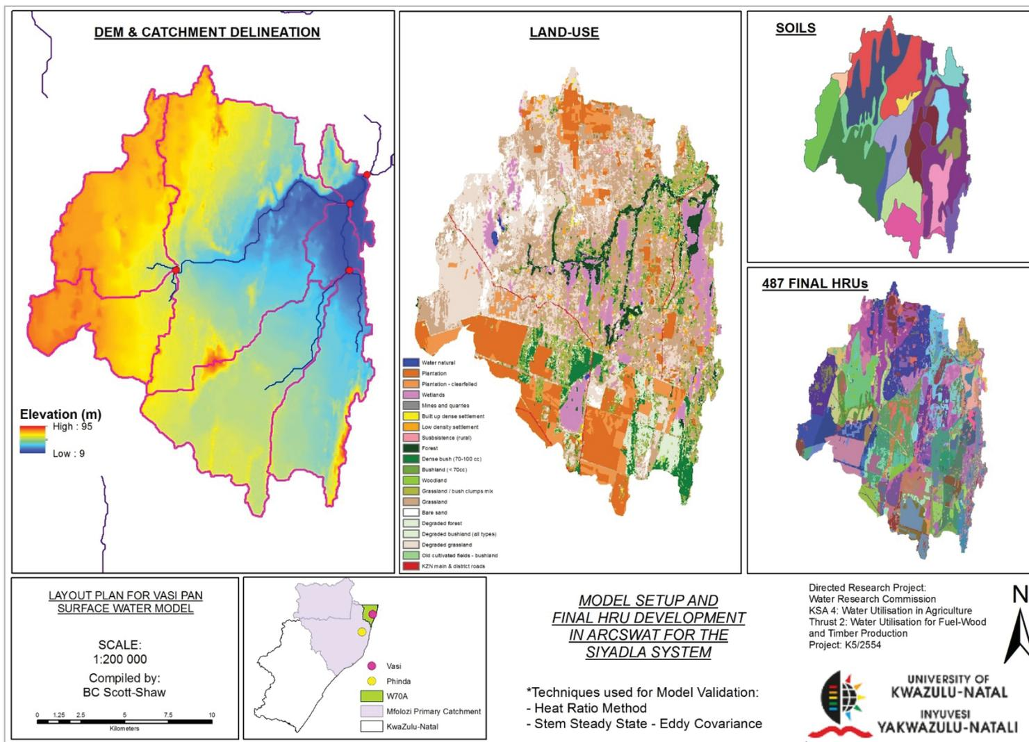
Figure 5.13 Set-up of the Vasi Pan catchment using ARCSWAT
