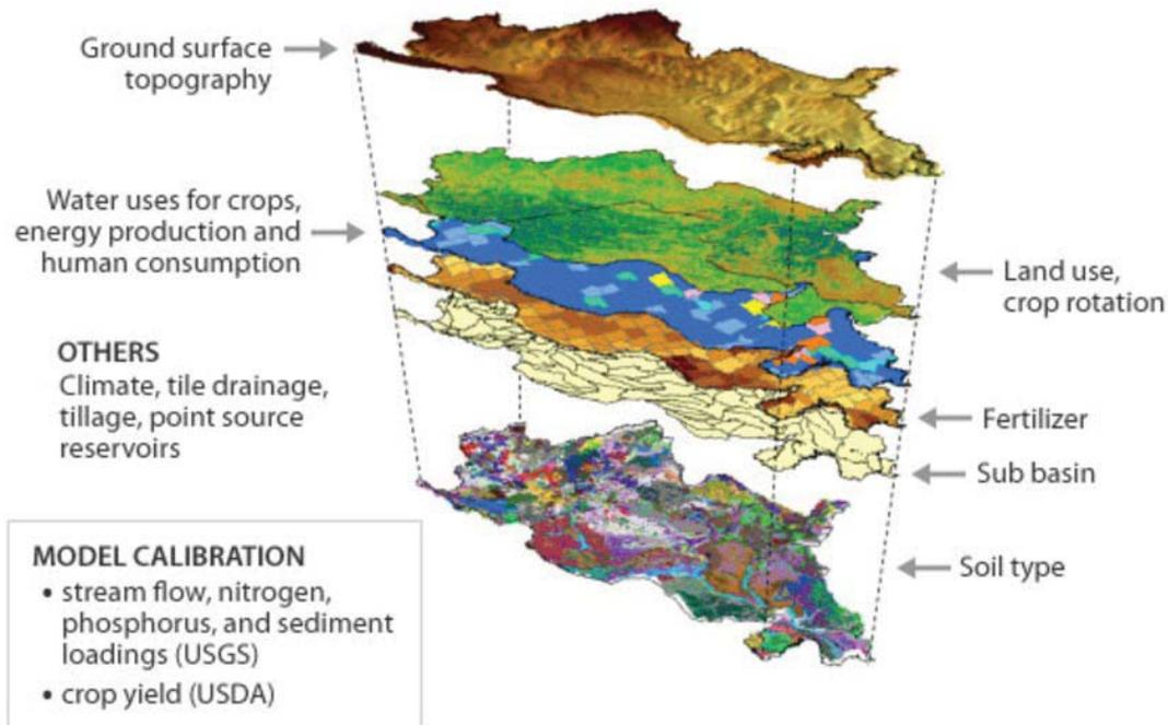
Figure 2.9 Conceptual layout of the ArcSWAT model setup
