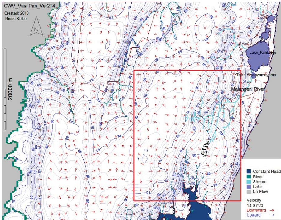
Figure 6.32 The simulated water table elevation contours (mMSL) for the Regional Model. The red arrows indicate the flow direction that is perpendicular to the head contours.
