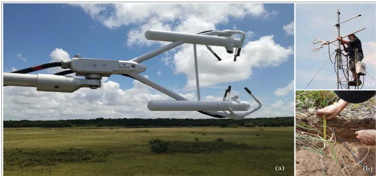
Figure 5.7 Equipment installation of the eddy covariance system in Vasi Pan. a) IRGASON (Campbell) placed on the mobile EC system in the hygrophilous grassland; b) placement of Soil Heat flux plates and Soil Thermocouple probes; c) installation of EC150 CO<sub>2</sub> and H<sub>2</sub>O open path gas analyser on the lattice mast in the indigenous forest
