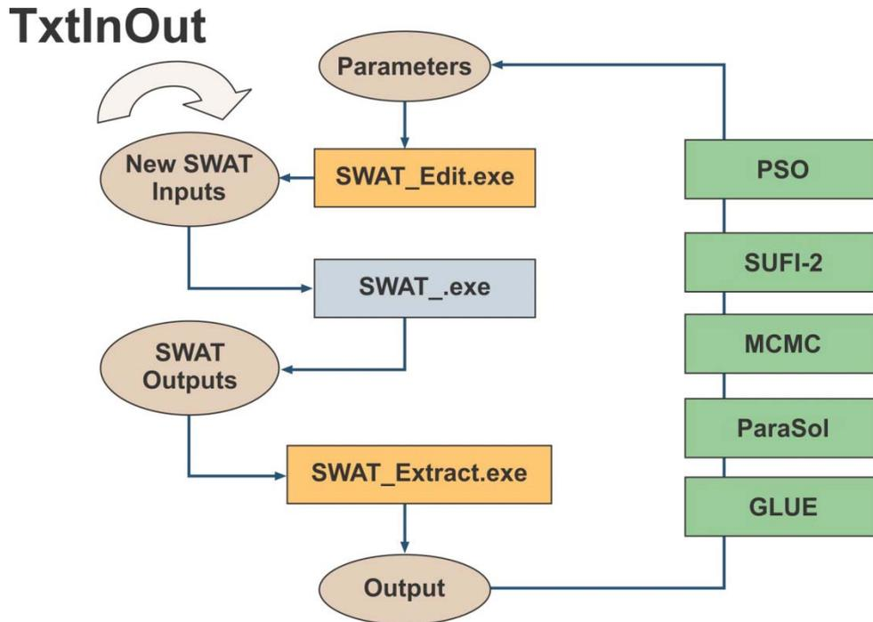
Figure 5.14 SWAT-CUP process for the optimization of the models (Abbaspour, 2015)
