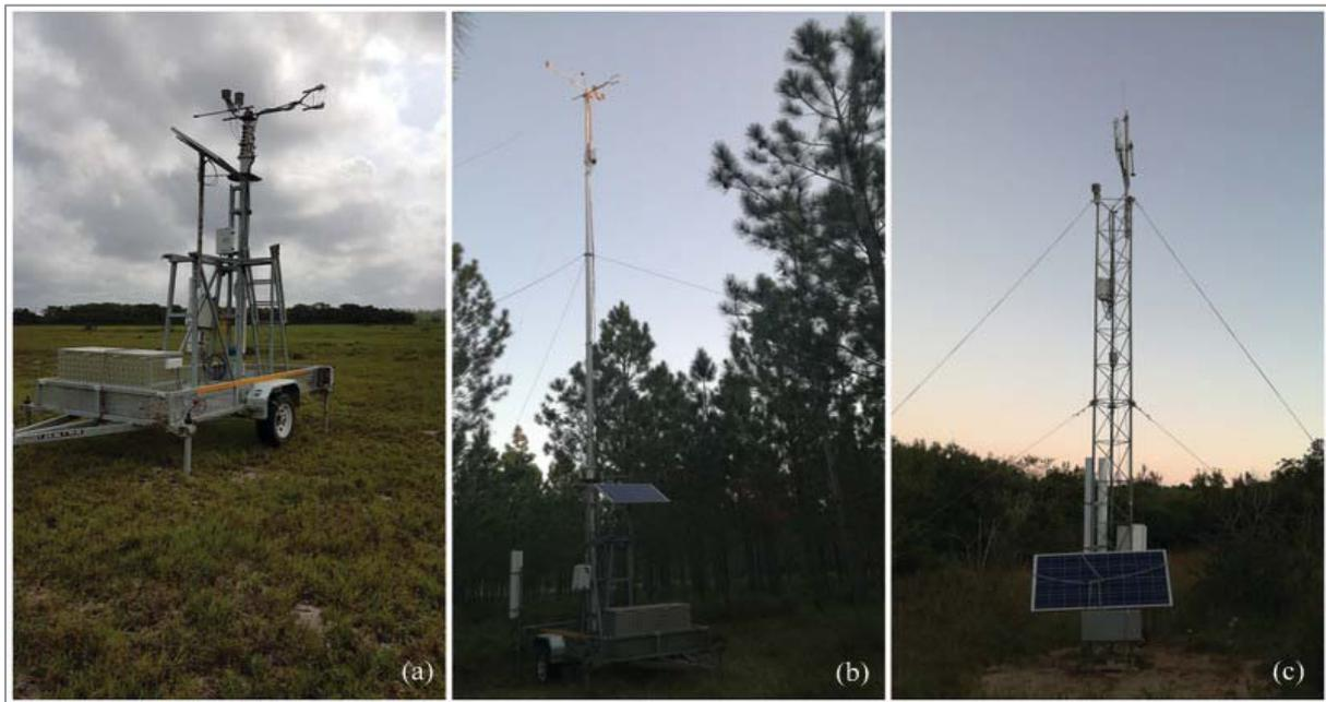
Figure 5.8 Selected EC monitoring sites: a) trailer system in the hygrophilous grasslands; b) trailer system monitoring a commercial pine stand; c) permanent lattice mast in indigenous forest
