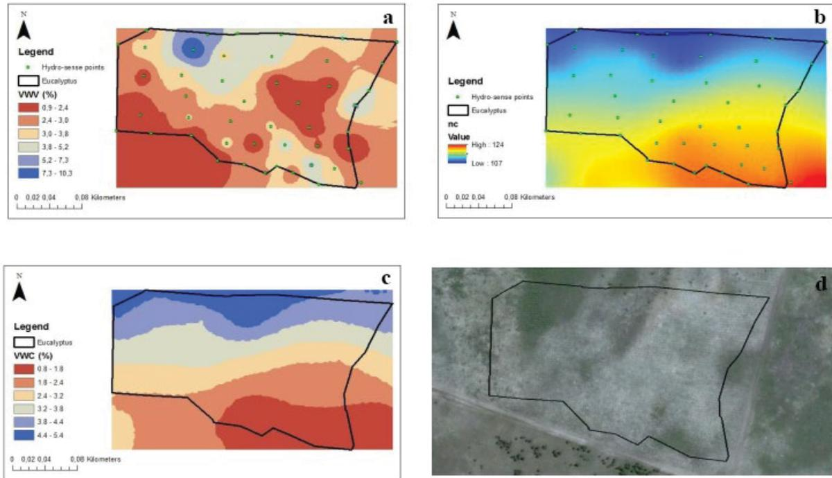
Figure 6.24 Maps of the Hydro-sense measurements (a), corrected neutron counts (b), cosmic ray rover estimates (c) and landcover (d)
