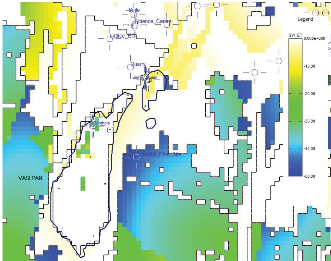
Figure 6.38 The simulated rate of evapotranspiration ( $10^{-1}$ mm/day) from the saturated zone for each  $100 \times 100$  m cell. The black lines are the different land use zones. The scale shows the groundwater evaporation in units of  $\text{m}^3/\text{day}$  from an area of  $100 \times 100 \text{ m}^2$ .
