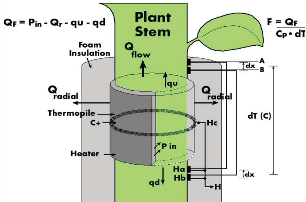
Figure 3.12 Sap flow sensor operation and the calculation of sap flow
