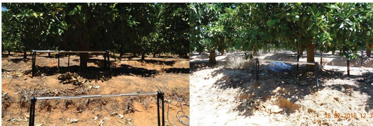
**Figure 3.16 Tube solarimeters used to continuously measure solar radiation received at the orchard floor**
