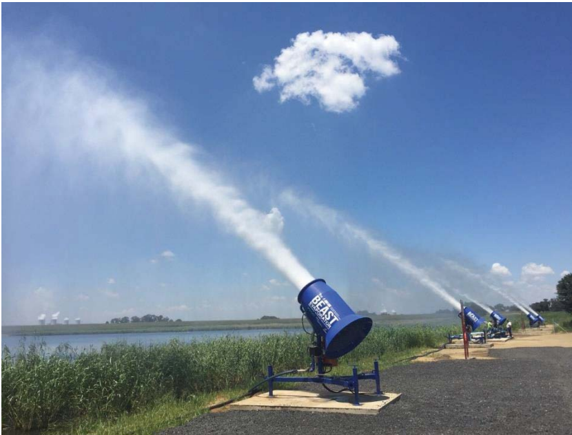
Figure 36: Mechanical evaporator equipped with a booster pump
