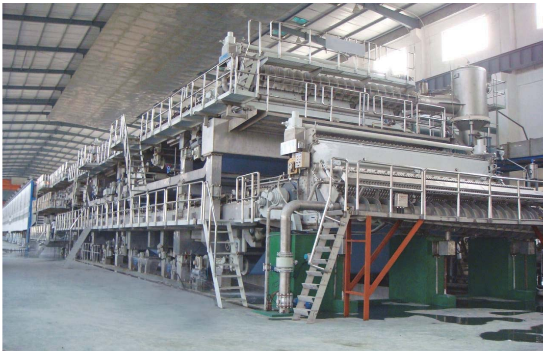
Figure 83: Following Unplanned Load Shedding Paper Machines need to be washed out before re-start
