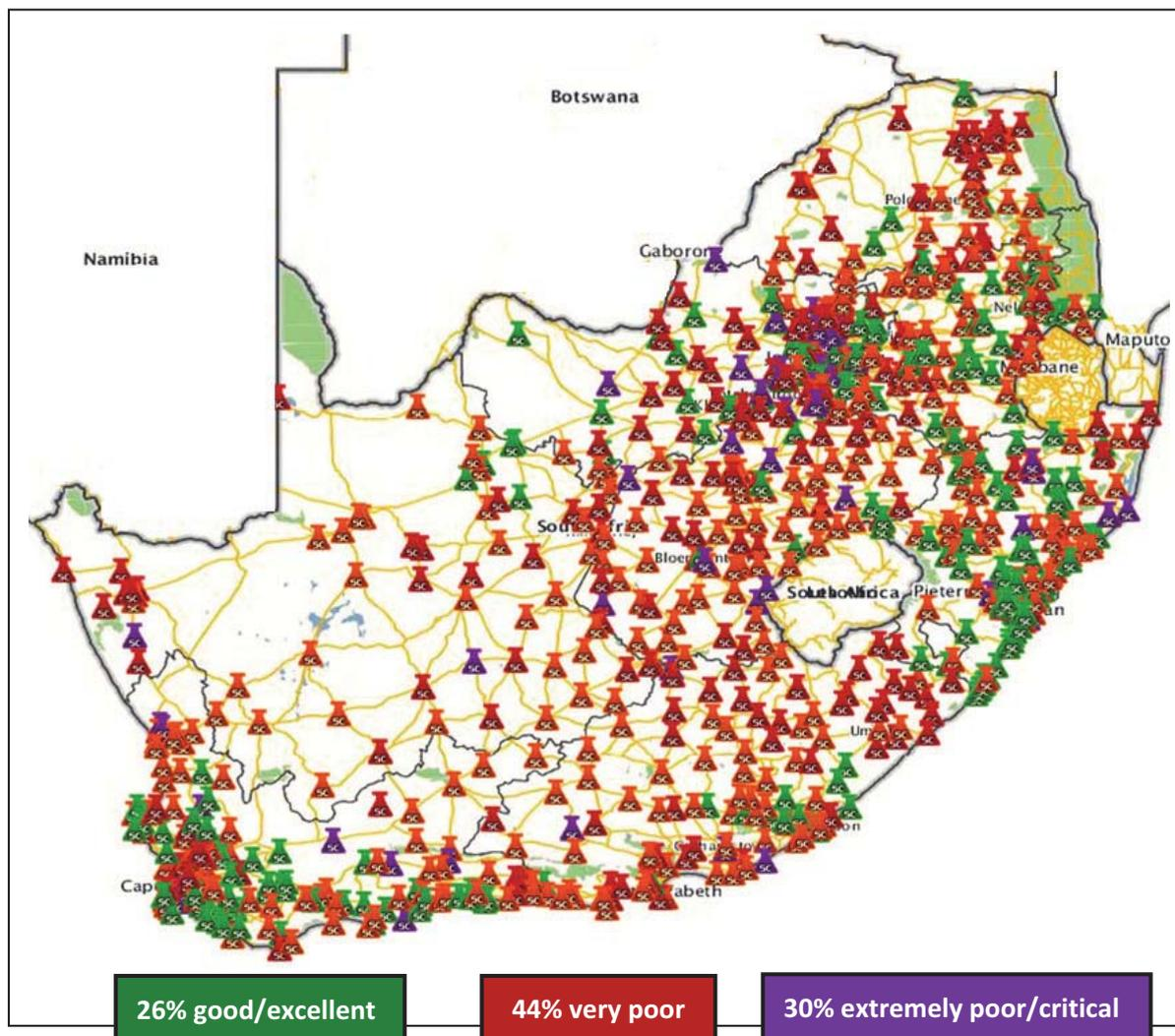
**Figure 7:** Performance rating of wastewater treatment works in South Africa based on extent of exceeding capacity, effluent compliance, skills deficit and delivery functionality (DWA, 2012)
