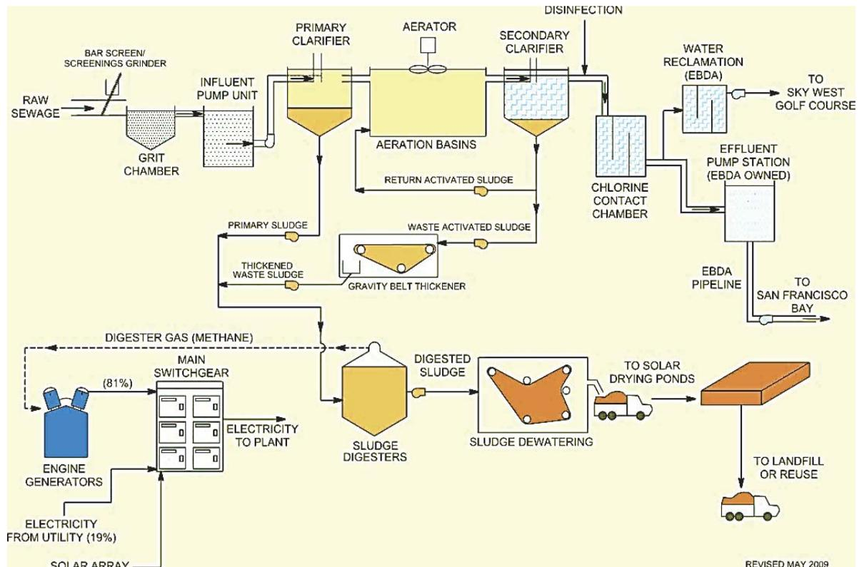
**Figure 18:** A schematic of the components and process of a wastewater treatment system
