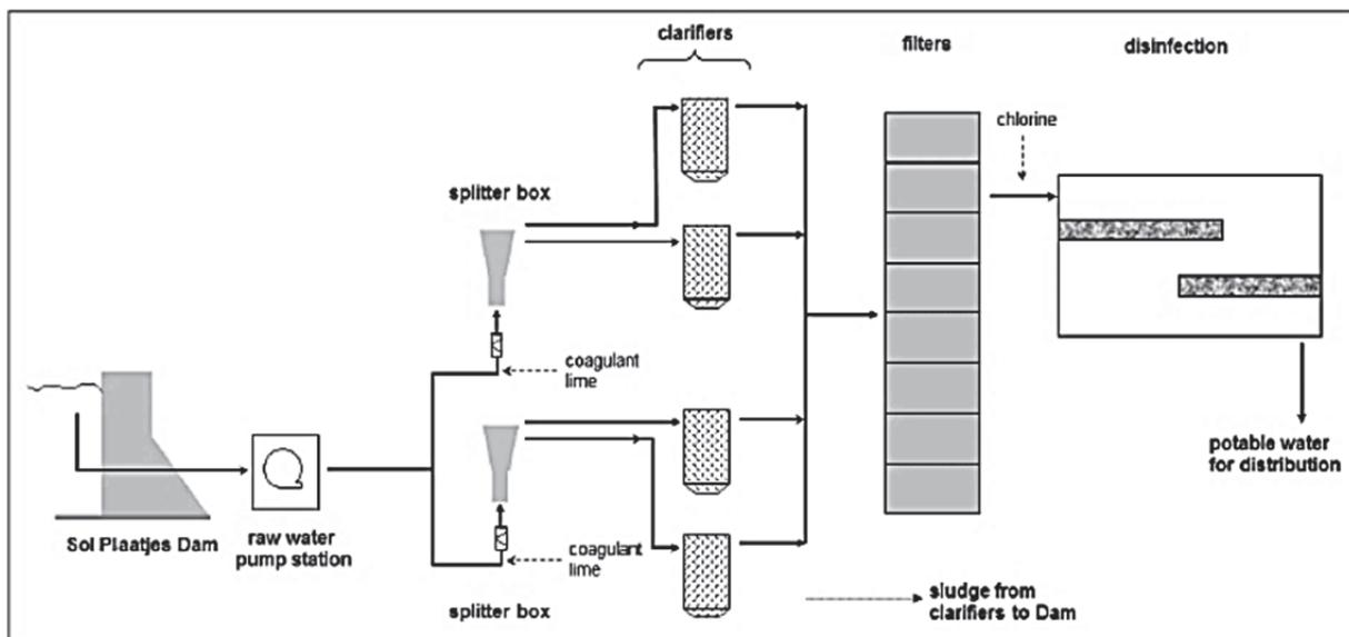
**Figure 17:** The schematic of a typical water treatment works for a municipality in South Africa. (Source: Budhram et al., 2013)
