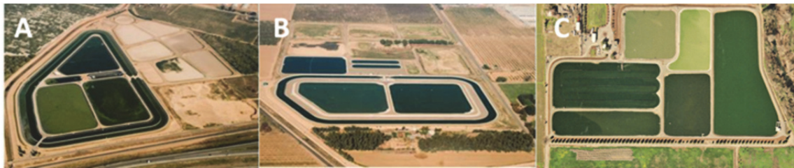
Figure 2 Examples of IAPS implemented in California, USA. A) Delhi, California: design flow = 3.2 \text{ M}\ell\cdot\text{d}^{-1} , wet surface area = 8 ha, total area = 16 ha; B) Hilmar, California: design flow = 2.5 \text{ M}\ell\cdot\text{d}^{-1} ; wet surface area = 7 ha; total area = 15 ha; C) St Helena, California: design flow unknown.
