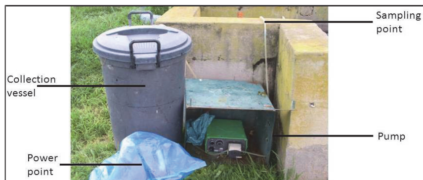
Figure A.1 Setup for collection of a composite sample using a standard municipal dustbin over a 24 h period.
