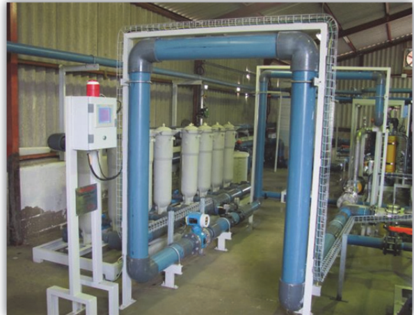
Pressure exchanger energy recovery system (part 80%)
