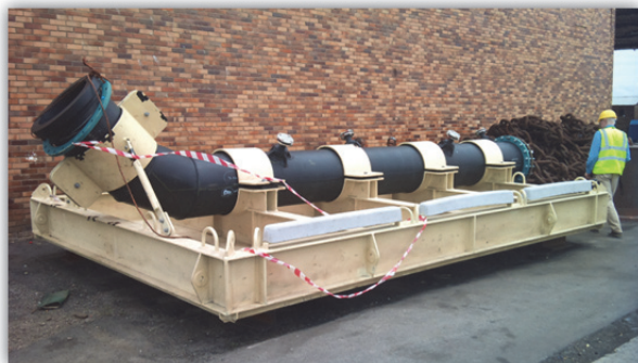
Brine discharge to sea with diffuser 450m offshore
