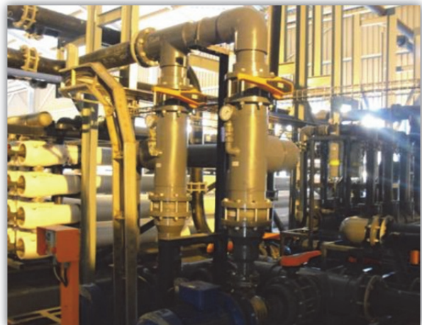
RO cartridge filters, pressure vessels and pipework
