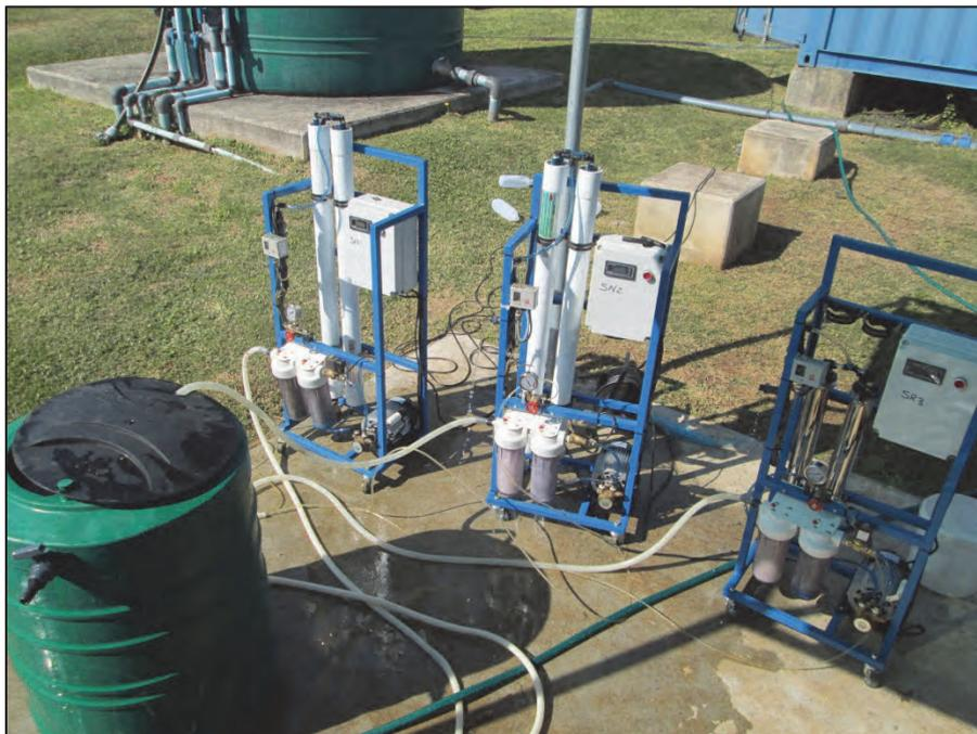
Figure 2.10: RO Membrane Test Rigs Operating in Parallel
