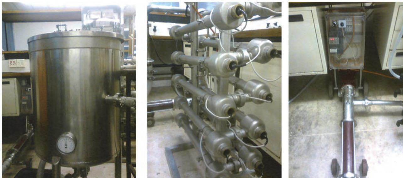
**Figure 2.12: UV Pilot Unit showing: Recirculation Feed Tank, UV Lamps (x10) and Pump**
