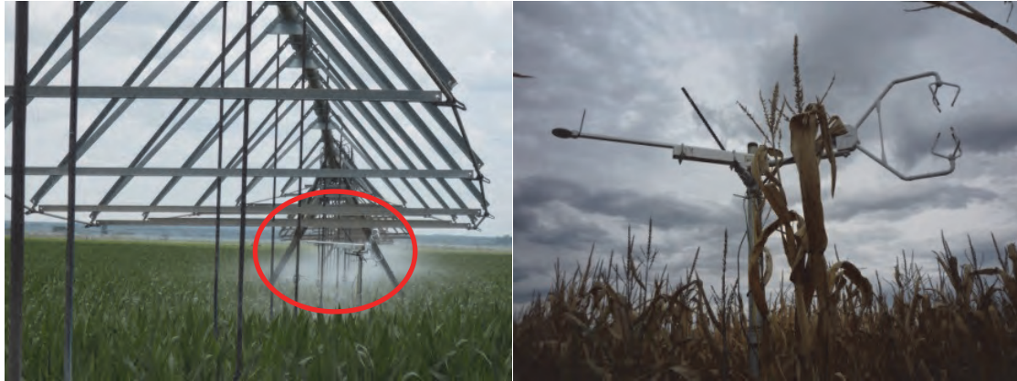
Figure 35. One sensor eddy covariance system with CSAT-3 sonic anemometer installed close to the centre of a pivot planted with maize. The EC system is here shown at full canopy cover as the pivot moves over it, and prior to harvest.
