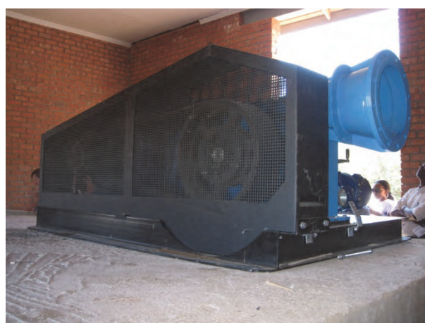
Figure 10-22: Crossflow turbine (belt driven)
