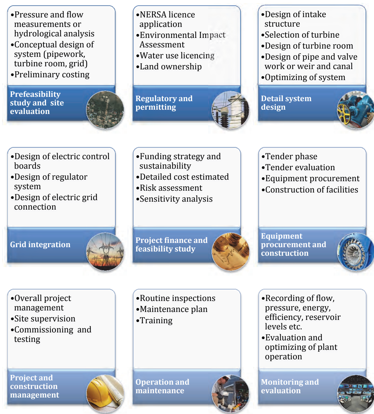
Figure ii: Conduit hydropower development process diagram
