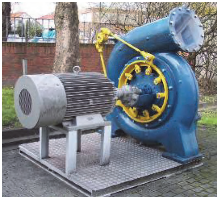
Figure 2-29: Loring road Francis turbine (200 kW)
