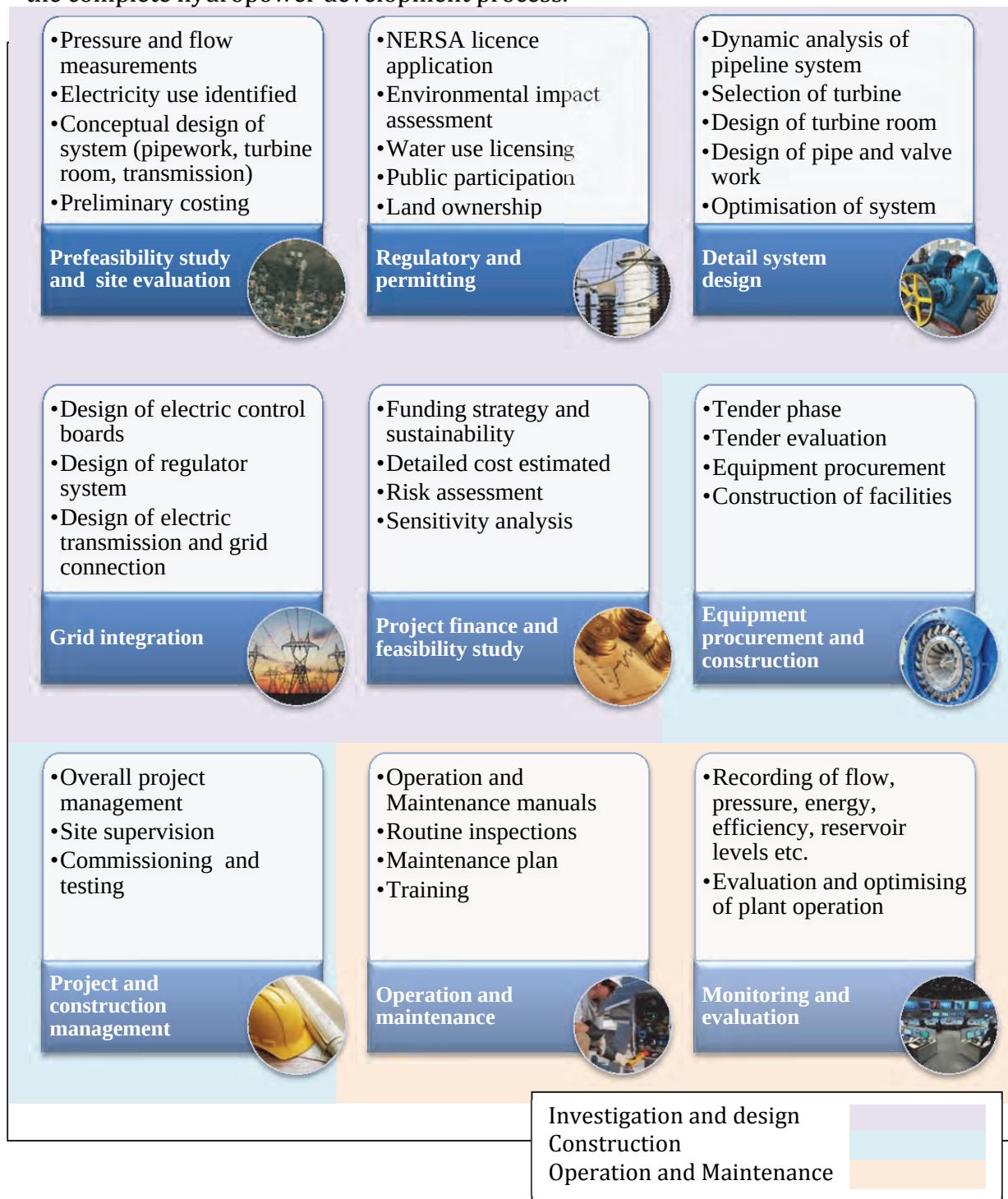
Figure 6-1: Conduit Hydropower Development Scope of Works
