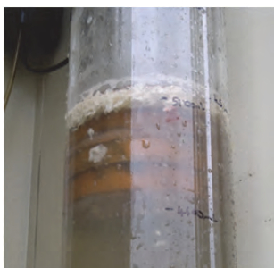
Figure 73: Inoculating the AGS reactor with the biofilm grown in the lab.
