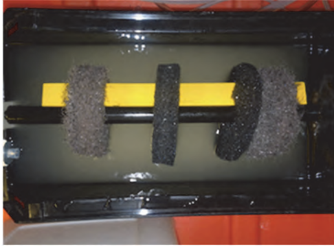
Figure 64: At substrate concentrations greater than 6 g/L, most of the biomass is still in the liquid medium.
