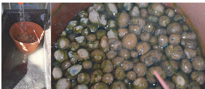
Figure 82: Examining the growth on a trickle bed setup with LECA balls and raw sewage.
