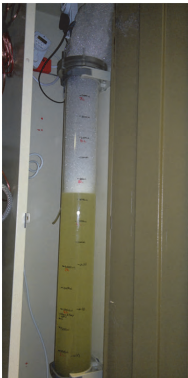
Figure 60 : Inoculated AGS reactor with synthetic media (6 g/L substrate) displaying excessive foaming.
