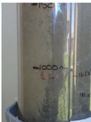
Figure 72: Very fluffy growth on sides of reactor.
