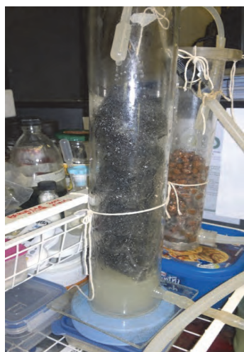
Figure 80: A trickle bed reactor with two support media alternatives, inoculated with synthetic media and Isolate 1 : To the left is the mesh used in the RBC, and to the right is a lightweight expanded clay aggregate ('LECA balls').
