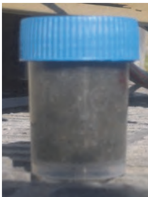
Figure 71: Sample of sludge. No granules visible. Note the reduced, black, 'anaerobic' nature of the sludge.
