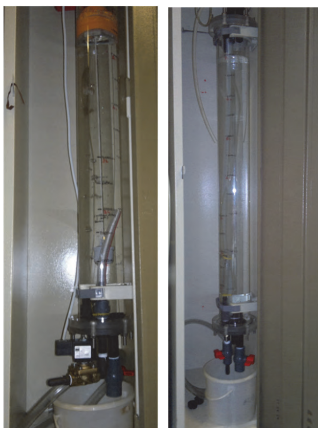
Figure 52: Aerobic Granular Sludge laboratory reactor setup constructed in this project.
