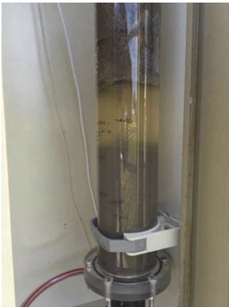
Figure 66: The AGS reactor with activated sludge build up at bottom of reactor.
