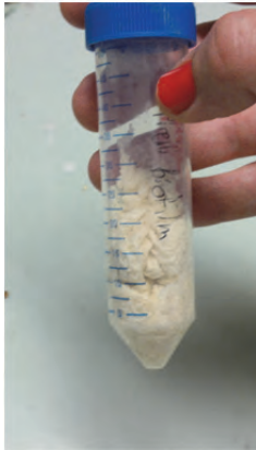
Figure 59: Biofilm harvested from a 100 mL shake flask to be added to reactors containing real wastewater
