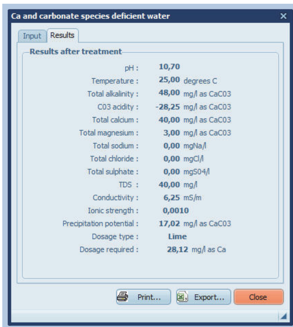
Figure 52: The results after treatment window for Example 11 (lime dosing).
