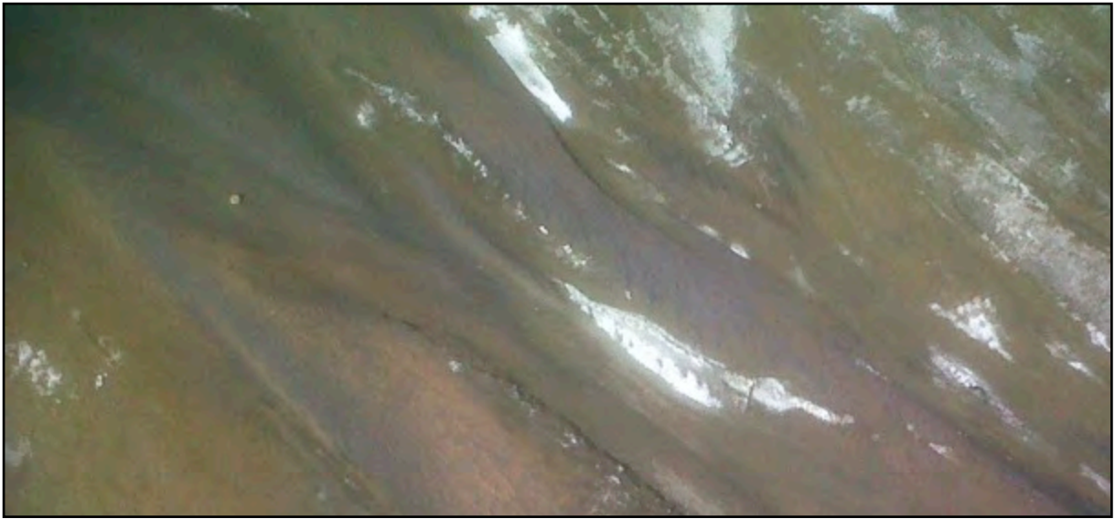
Figure 12-6. Precipitation of salts due to metals reacting with acidic seepage through the tailings.
