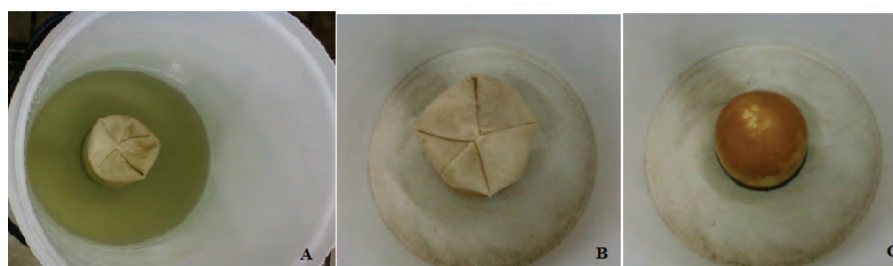
Figure 4.2: Photographs of stained ceramic candle: A – filtration of high-turbidity water; B – dirty jacket of candle filter after filtration; and C – clogged/dirty candle filter
