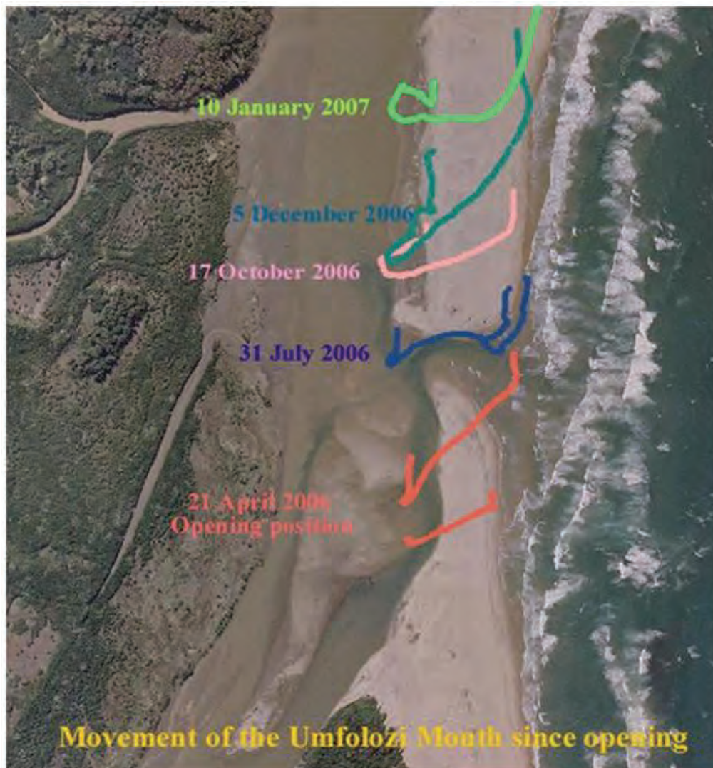
Figure 46. Regular mapping of the north bank of the Mfolozi Mouth using a GPS shows how it advanced northwards at a constant rate.
