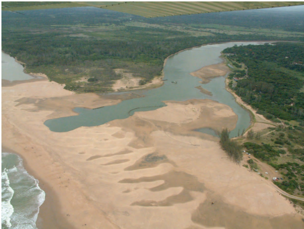
Figure 24. Dredging of the sediment trap. Note how the dredge was eating into the beach berm. Spoil was deposited on the beach in front of the car park ( 22 December 2003, R Taylor).
