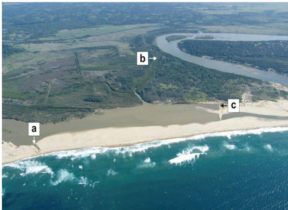
Figure 63. The plan to activate the Back Channel was implemented – by closing the Mfolozi Mouth (c) and creating a “weak link” near Maphelane (a). The backing up Mfolozi water would flow via the Back Channel (b) into St Lucia.
