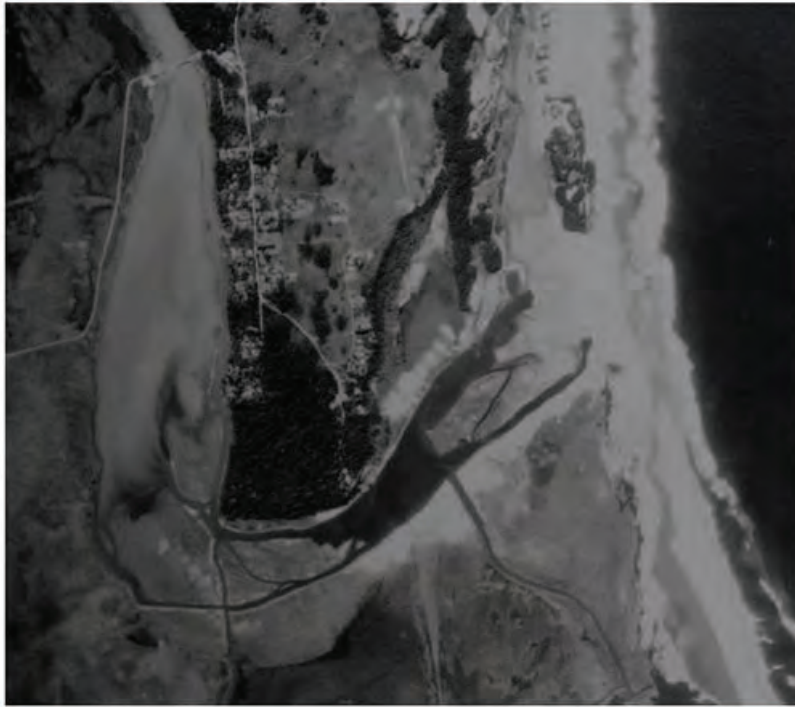
Figure 2. Aerial photograph of the St Lucia mouth taken in 1960 showing the extent of the dredge operations that had started in the mid-1950s. It also shows the extent of the remaining sediments.
