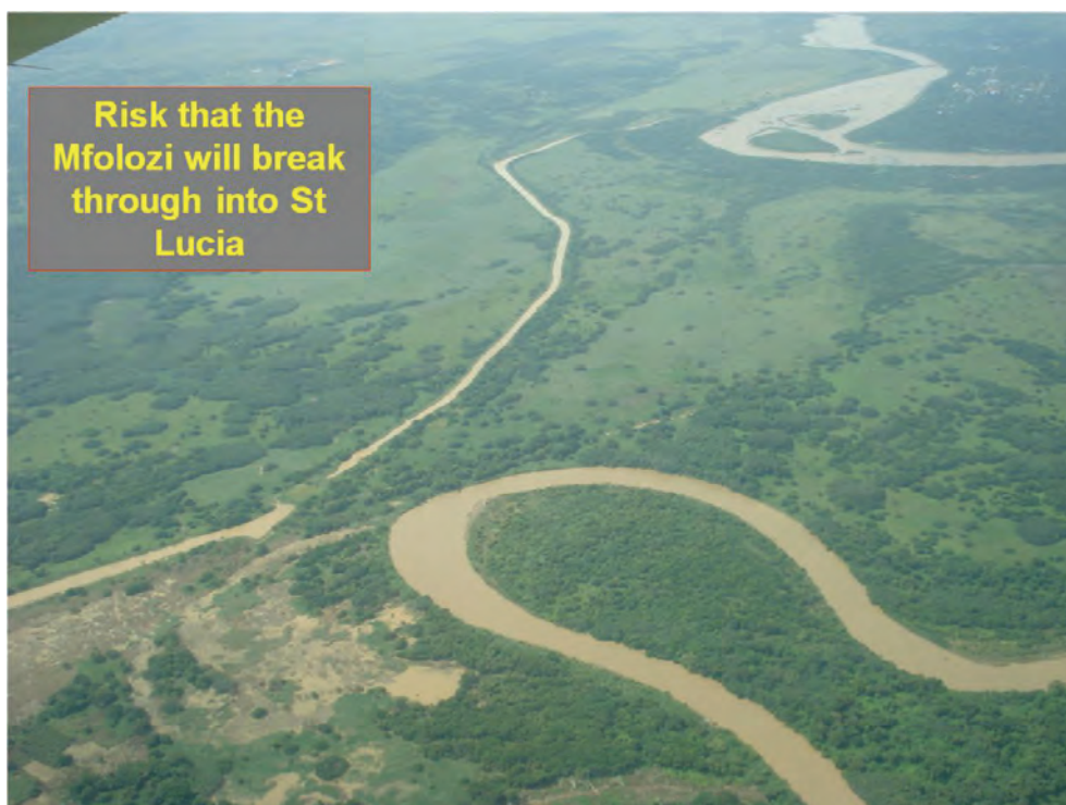
Figure 72. After the flood had again overtopped into the Link Canal there were concerns about the Mfolozi River taking this as a permanent route. The Link Canal is in the upper left of the photo, the meander in the Mfolozi River in the bottom right and the St Lucia Estuary in the upper right.
