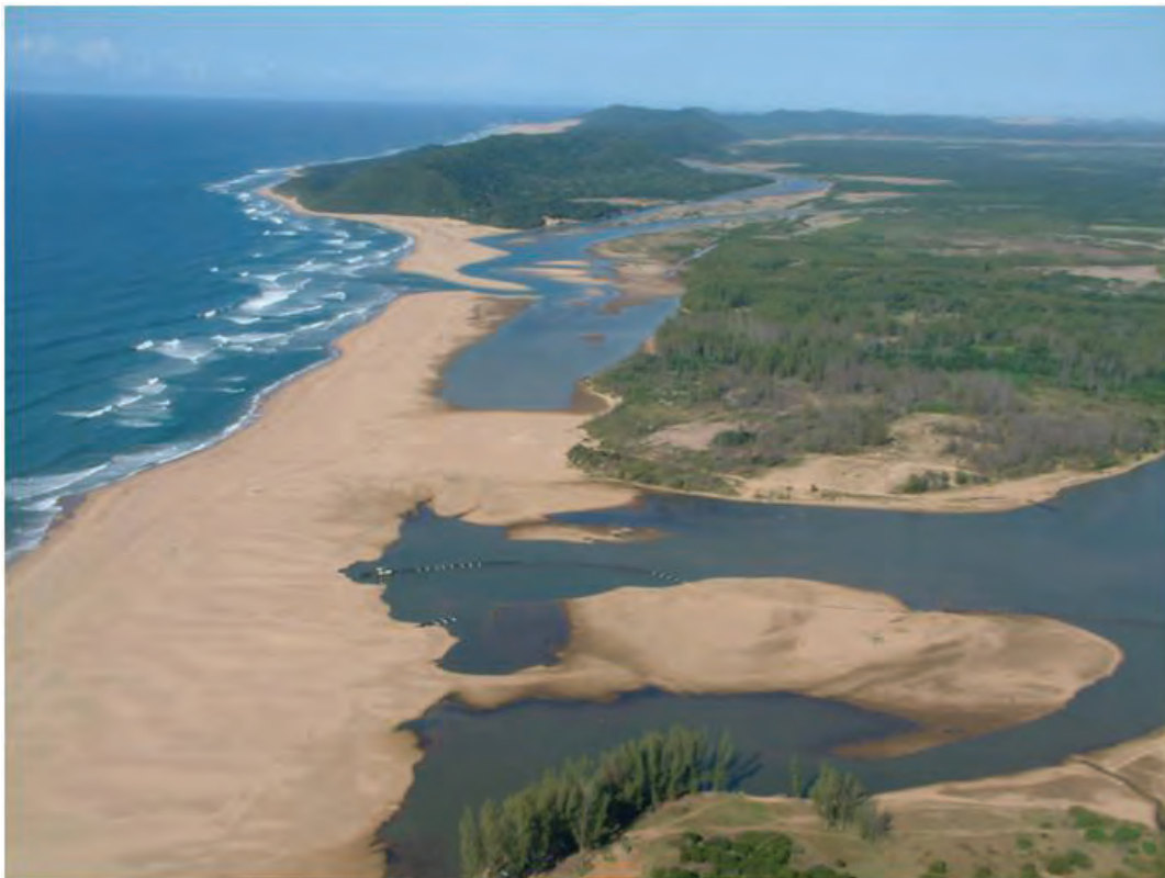
Figure 11. Configuration of the mouths in May 2003 showing the closed St Lucia Mouth in the foreground. The dredge was excavating the sediment basin at the time, pumping the spoil northwards.
