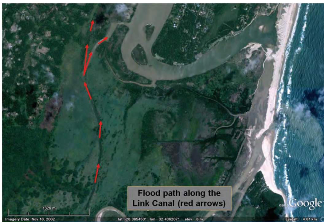
Figure 101. The path for flood waters that overtop from the Mfolozi River during flood events. This water passes into Honeymoon Bend.
