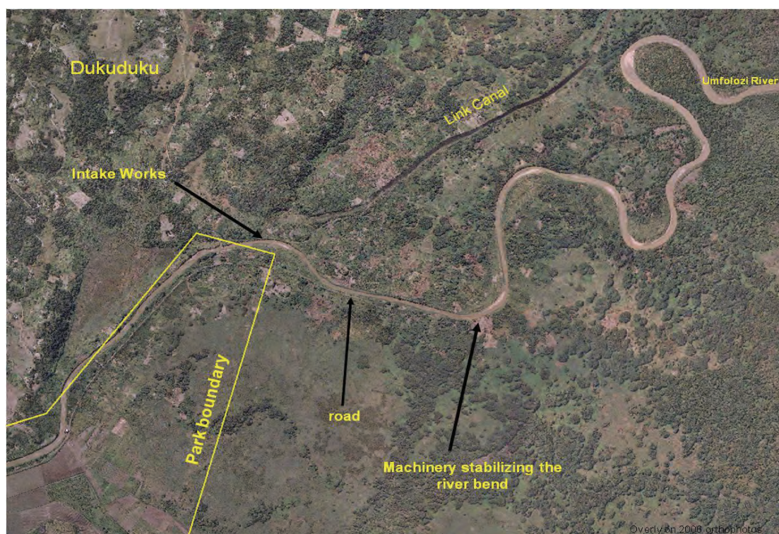
Figure 55. The UCOSP had been building up the south bank of the Mfolozi River to prevent it from breaching southwards and flooding sugarcane fields. This action prevents the southward channel switching of the river.
