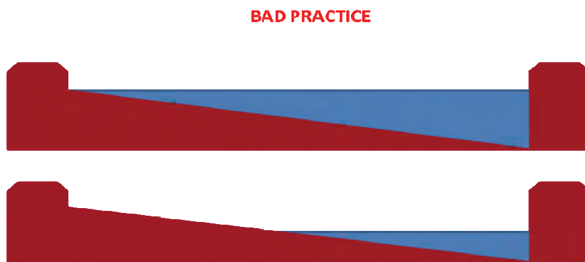
FIGURE 2: When the furrow bottom has a slope, water will disappear first in the upper part and only later on in the bottom part
