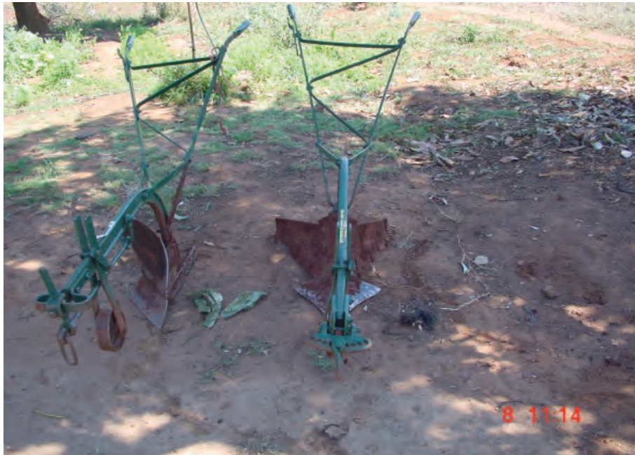
PLATE 5.1: The VS8 single furrow plough and the high wing ridger supplied to participants at Dzindi and Rabali
