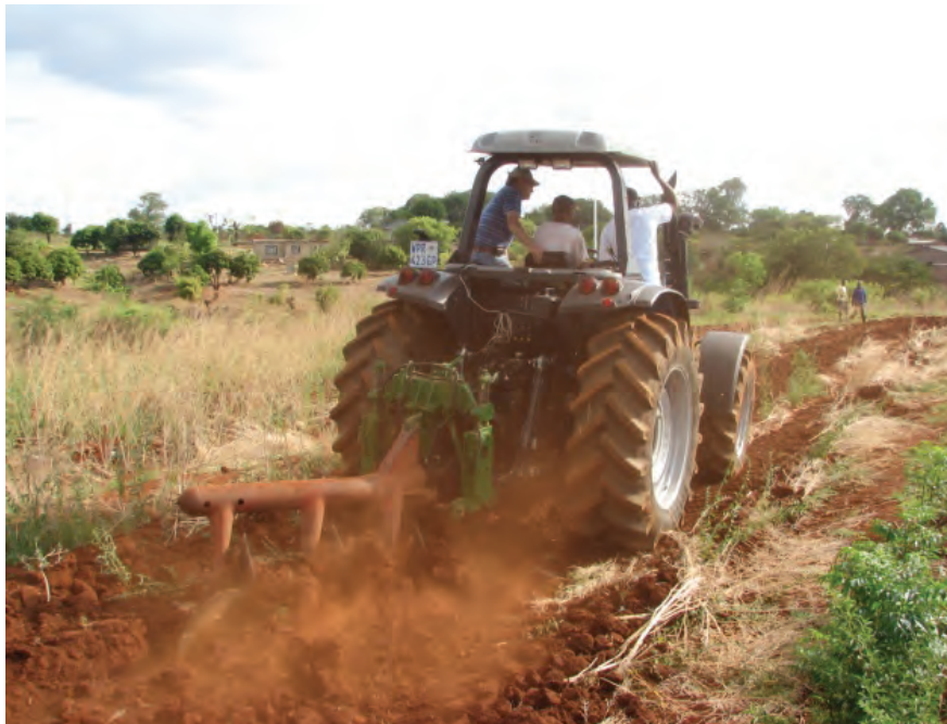
PLATE 5.4: A dynamometer was attached between the tractor and implement on the linkages to measure draught and power output
