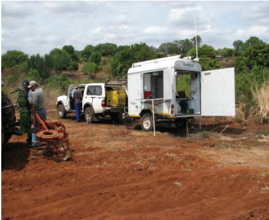
PLATE 5.3: Telemetry was used to collect data on measure draw bar power required to pull the tractor drawn implements
