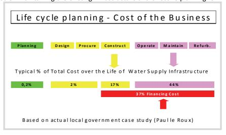
considering the lifecycle cost of typical wastewater infrastructure (F van Zyl, 2006), it is noted that <20% of total cost is tied up as initial capital, whilst 44% of the lifecycle costs is in operations and maintenance, which must be recovered from the municipal tax base.
