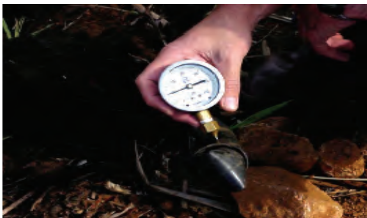
Figure 14. Pressure measurement in the lateral 9)
