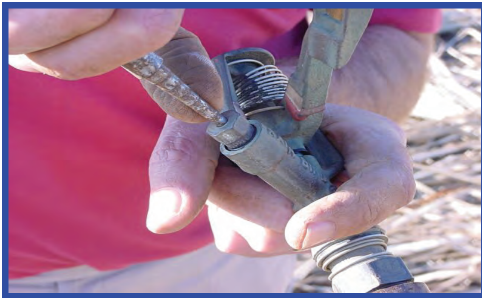
Figure 9. Measuring device for sprinkler nozzle size (Source: F Reinders)
