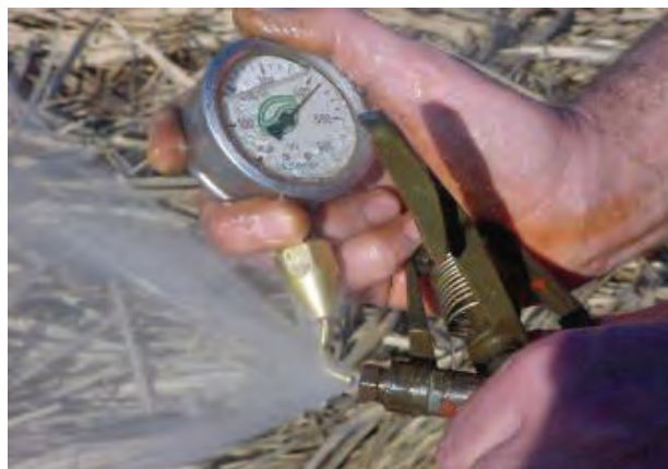
Figure 5. Measuring of operating pressure of sprinkler irrigation system
