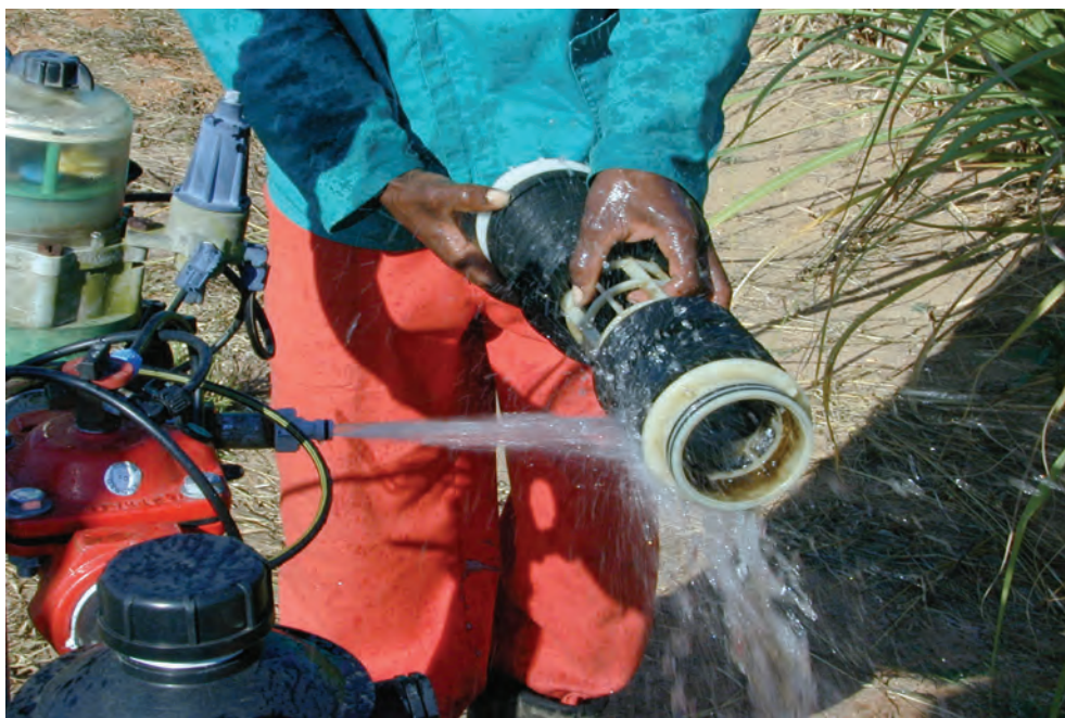
Figure 11. Spraying filter rings with high pressure water
