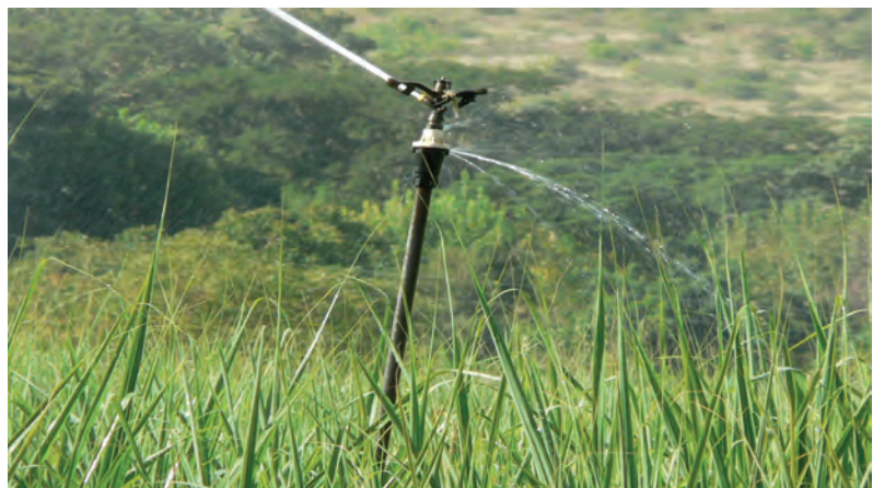
Figure 3. Sprinkler with leaking pressure regulator
