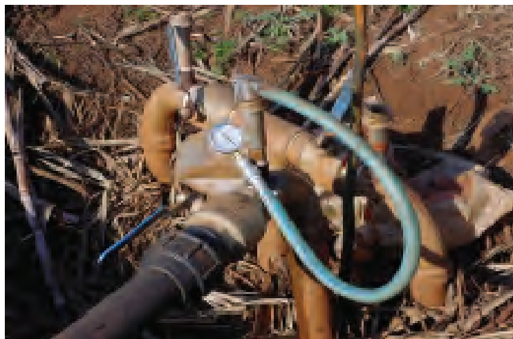
Figure 13. Pressure measurement at hydrant 9)
