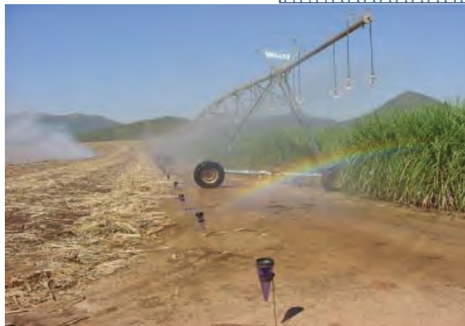
Figure 4. Measuring uniformity with rain gauges 9)
