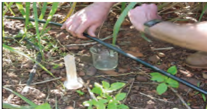
Figure 15. Discharge test of surface drippers (Source: F Reinders)
