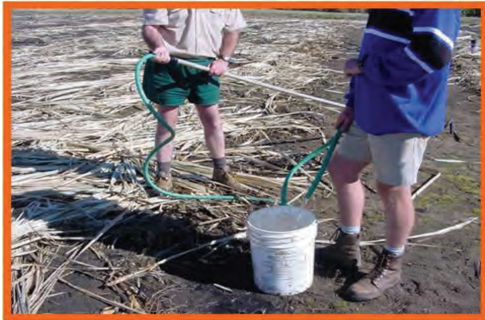
Figure 10. Measuring of sprinkler discharge 9)
