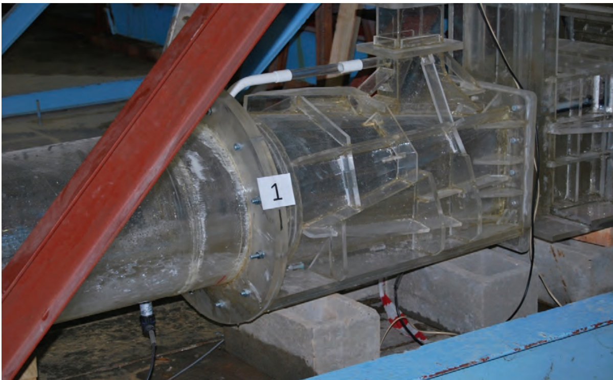
Figure 5-13 B: Flow pattern in emergency gate and air vent region for 20% emergency gate opening (Physical)
