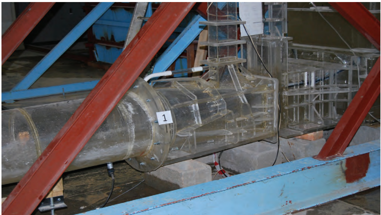
Figure 5.14 B: Flow pattern in emergency gate and air vent region for 30% emergency gate opening (Physical)
