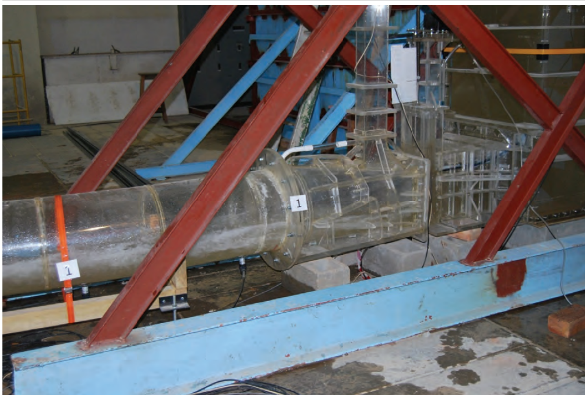
Figure 5.15 B: Flow pattern in emergency gate and air vent region for 40% emergency gate opening (Physical)
