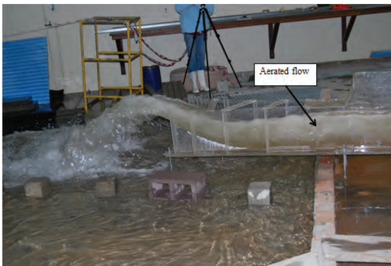
Figure 5-21 B: Flow pattern at ski jump and end box for 40% emergency gate opening
