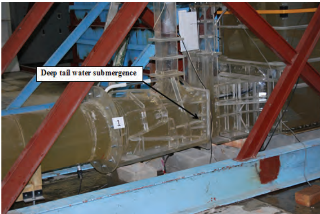
Figure 5-18 B: Emergency gate region on physical model for 70% emergency gate opening
