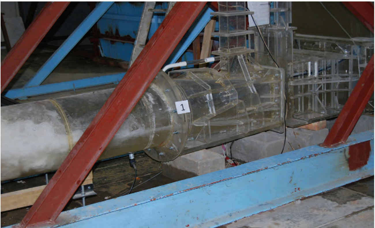
Figure 5-16 B: Flow pattern in emergency gate and air vent region for 50% emergency gate opening (Physical)
