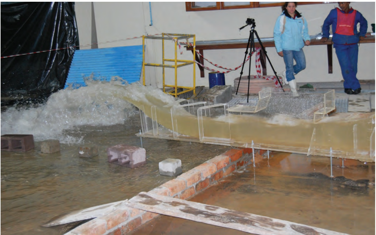
Figure 5-23 B: The ski jump for 60% emergency gate opening (Physical)
