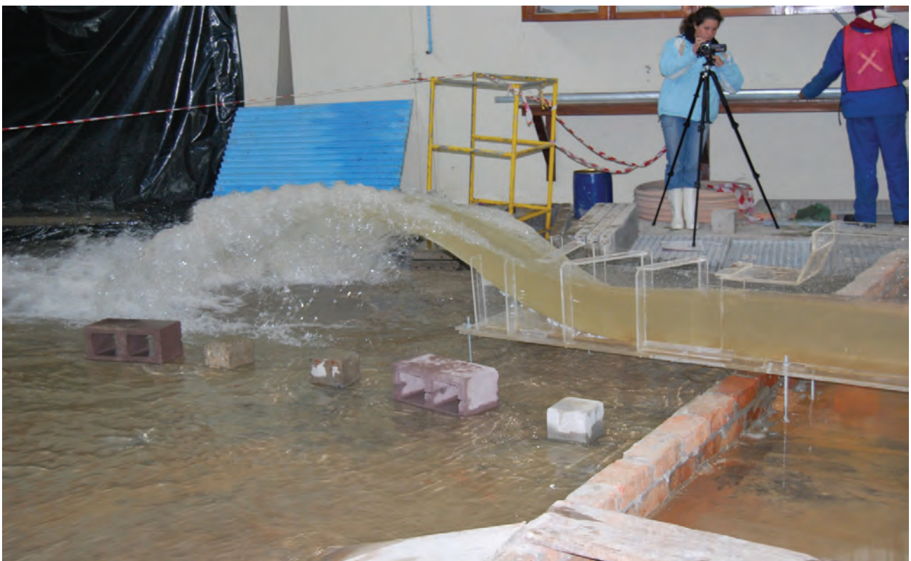
Figure 5-24 B: The ski jump for 70% emergency gate opening (Physical)
