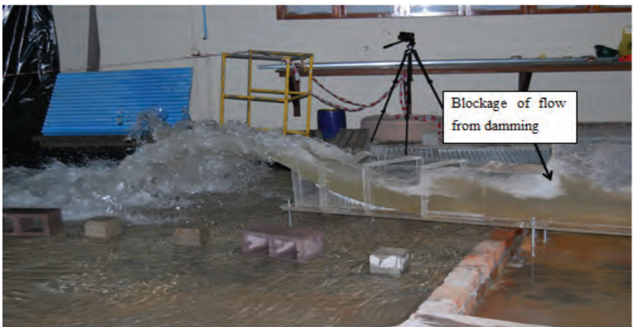
Figure 5-22 B: The ski jump for 50% emergency gate opening (Physical)
