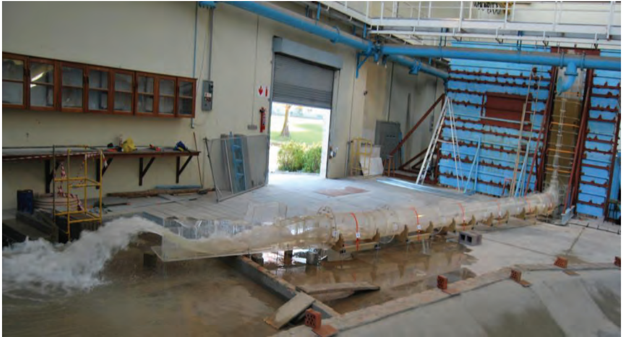
Photo 1: Layout of Berg River Dam Model
