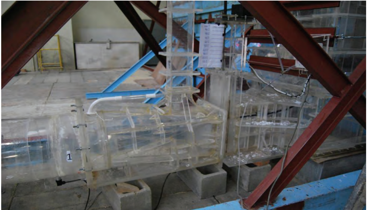
Photo 2: Emergency gate, base of air vent and outlet conduit
