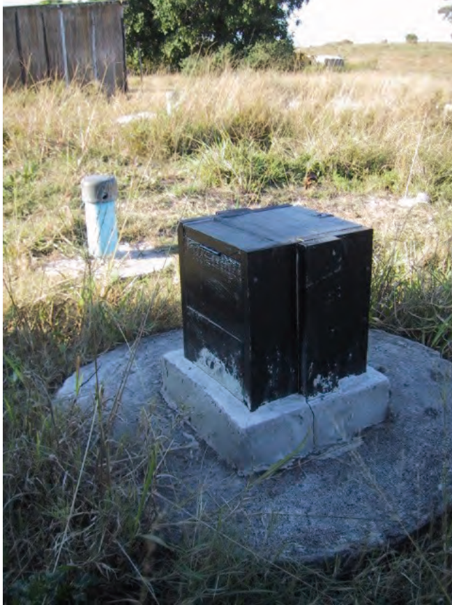
Figure 2: In the foreground a completely sealed off monitoring well can be seen. In the background the earlier version of the monitoring well can be seen. This was sealed with an end cap which was locked in place. However, it was later felt that the opening for the lock exposed the monitoring well to the risk of contamination (from, for example, small animals).
