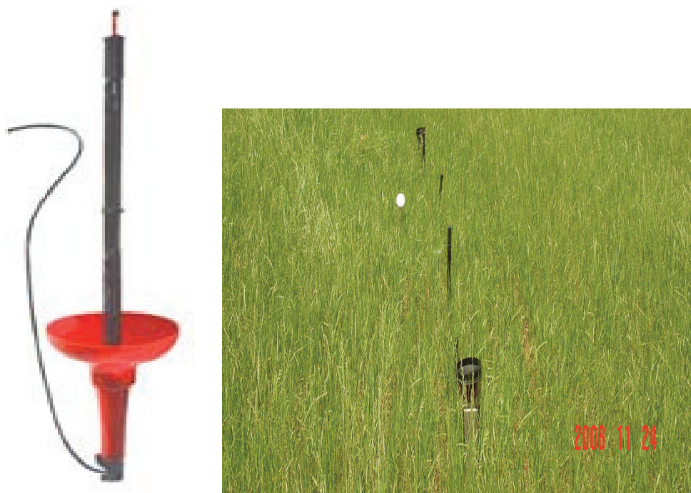
Figure 3 Wetting front detector (WFD) for managing irrigation and nutrients
