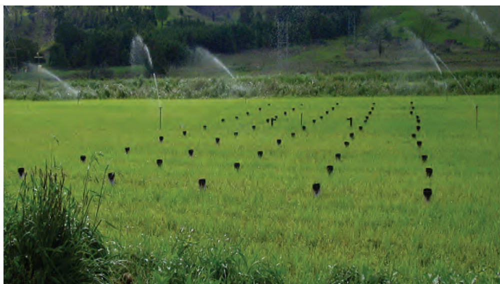
Figure 3.2 Layout of dragline sprinkler system and placement of raingauges for uniformity test of the dragline sprinkler irrigation system
