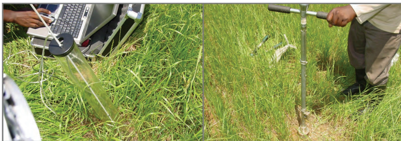
Figure 3.7 Minirhizotron soil tubes and root core sampler used for measuring root length and biomass
