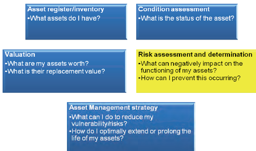
Figure 1: Key elements of Infrastructure Asset Management
