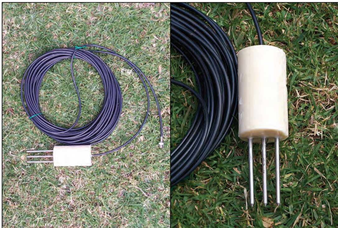
Figure 3.13. The design of the cylindrical TDR probes used for installation at depths > 2 m using an auger.
