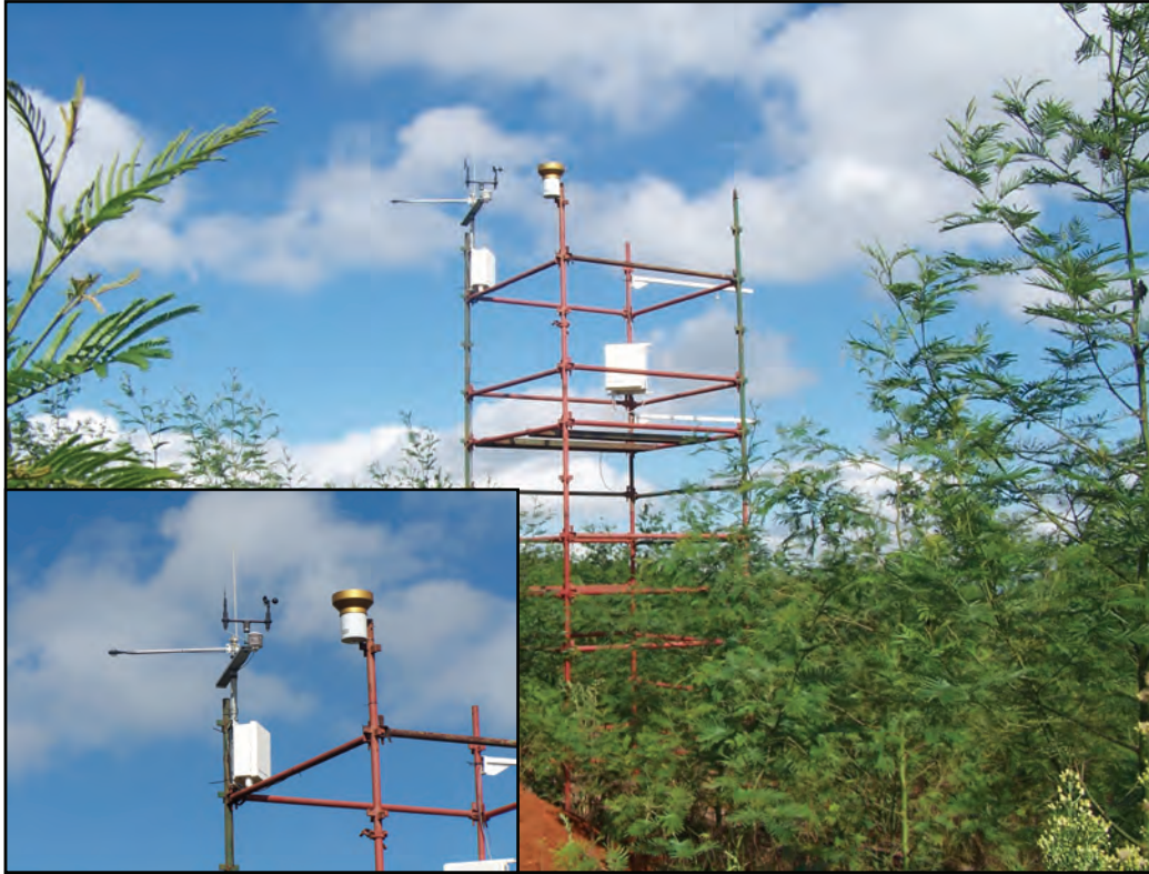
Figure 3.3. The above canopy automatic weather station in the centre of the wattle plantation used to collect net radiation and soil heat flux data as well as supporting meteorological data.
