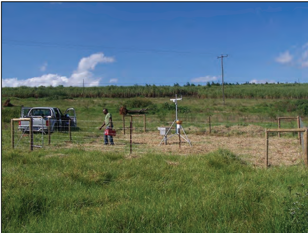
Figure 3.2. The automatic weather station near the Two Streams site established over short grass and used to calculate the short grass ASCE reference evaporation.
