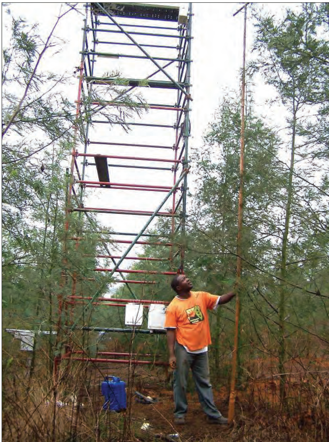
Figure 3.15. A soil auger with 1 m extensions was used to auger to a depth of 4.8 m.
