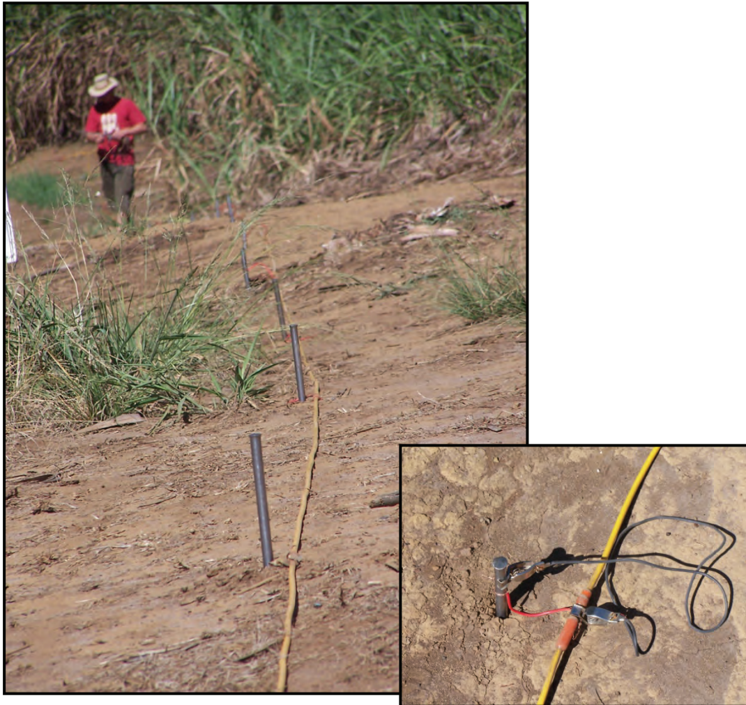
Figure 3.11. The cable and peg configuration used in the resistivity study.
