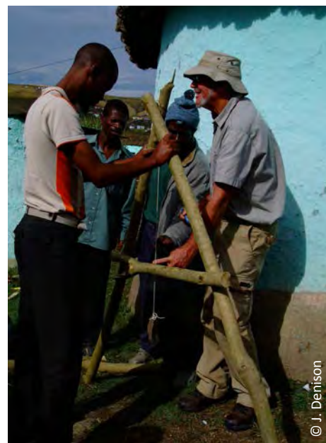
Figure 6.7 Calibrating an A-frame
