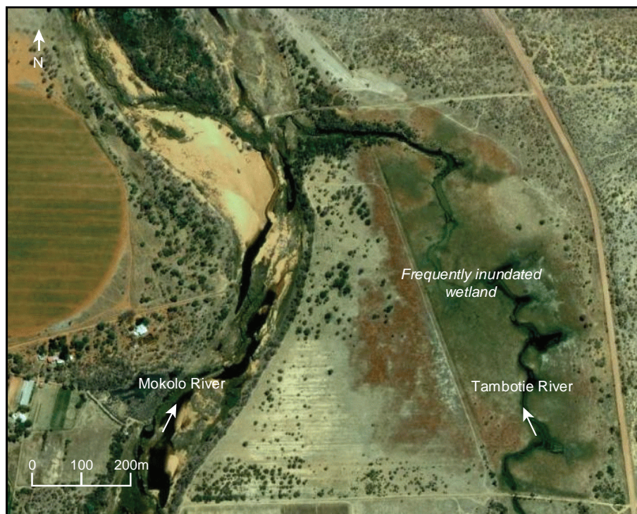
Figure 9-11 Annotated Google TM Earth satellite image of the Mokolo River floodplain system (23°47'38"S 27°46'00"E), showing the frequently inundated lower Tambotie floodplain resulting primarily from backup of Mokolo River flows. Flows in the Mokolo River are highly regulated by an upstream dam
