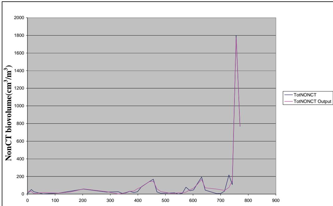
Figure 10 Results from the NeuroSolutions 5.04 ANN for the Non-CT producing group (TotNONCT), showing real time forecasting (pink line) versus the actual data (blue line).
