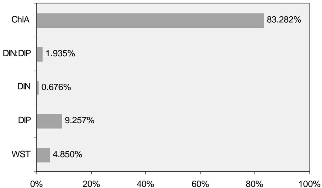
Figure 12 Percentage contributions of measured environmental parameters and Chl *a* concentration to ANN prediction for the Non-CT group in the Hartbeespoort Dam.
