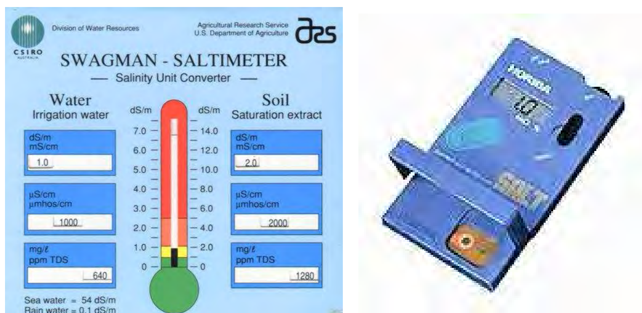
Figure 3.1. Left: The Swagman Salimeter (Meyer et al. 2004) Right: The Cardy Salt meter by Horiba
