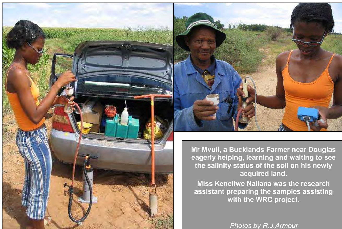
Figure 3.5. A possible infield ECe self-testing kit comprising of a soil bore, vacuum pump and filter (left) and on the right a close up of the salinity meter and probe inserted in the vacuum cup and the ceramic funnel and filter paper containing the saturated soil paste.
