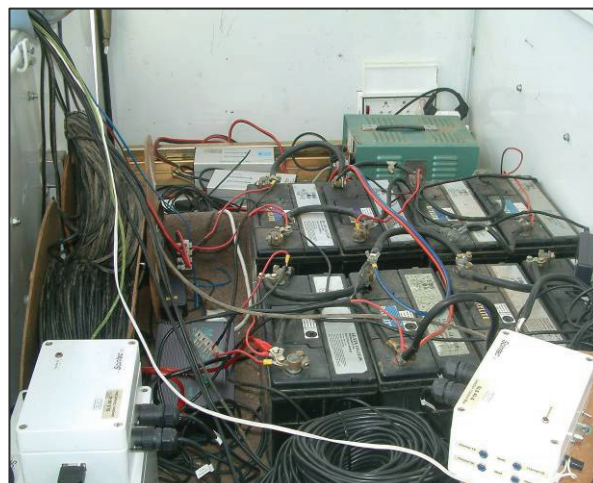
Plate 6.4. The specially designed petrol generator (left) and the battery chargers, invertors and two banks of four RR2 100 Amp hour batteries (right) used to power the two OEBMS1 systems.
