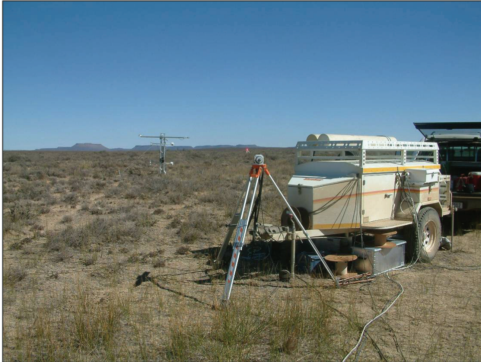
Plate 6.2. The setup of the dry veld OEBMS1 system (October 2007). The transmitter laser beam can be seen shining in the background.
