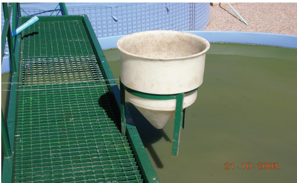
**Figure 4.1:** Funnel for feeding primary sewage sludge which was implemented following problems encountered with the continuous feeding system
