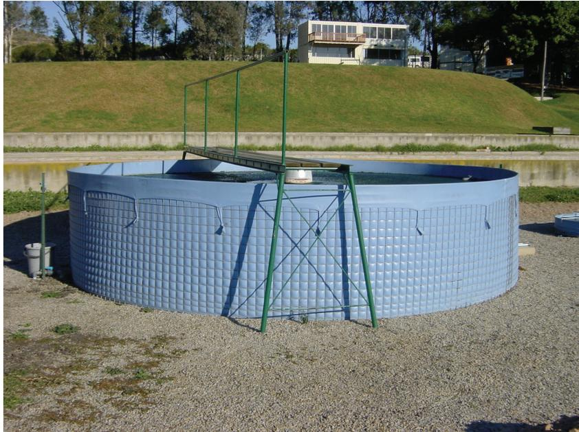
**Figure 3.6:** Advanced facultative pond constructed using a 5 m diameter porta-pool. The fermentation pit is located in the base of the pond.
