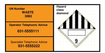
The vehicle carrying your wastes must display three of these placards: One on either side of the vehicle and one at the back. A truck and trailer combination with a waste container on the truck and containers on the trailer must display six placards in total.
