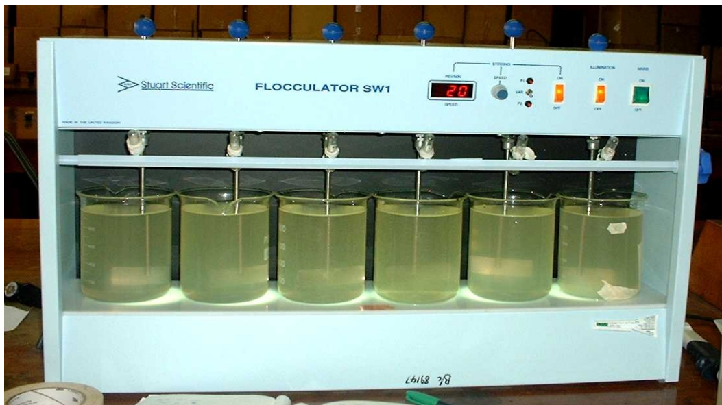
Jar test apparatus in use
