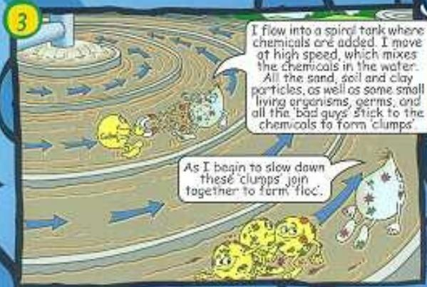
I flow into a spiral tank where chemicals are added. I move at high speed, which mixes the chemicals in the water. All the sand, soil and clay particles, as well as some small living organisms, germs, and all the 'bad guys' stick to the chemicals to form 'clumps'. As I begin to slow down these clumps join together to form 'floc'.
