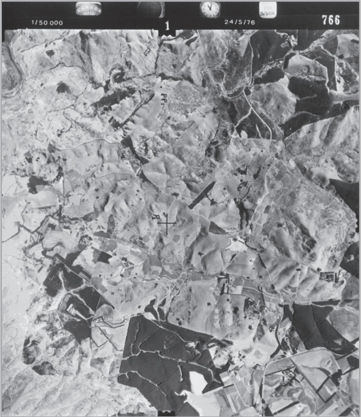
Figure A1.2: A contact aerial photo showing (L to R) approximate scale, strip no., date of photograph, photo no., and in the middle the Principle Point y.
