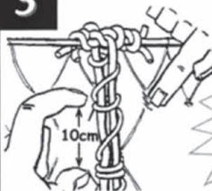
Secure the binding wire at the top corners of the panels. Lace the edges with single loops and double loops in turn, with 10cm. between them.
