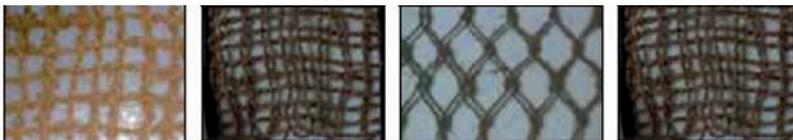
Figure 6.10: Different fibre netting types and densities ([www.erosionblankets.com](http://www.erosionblankets.com))
