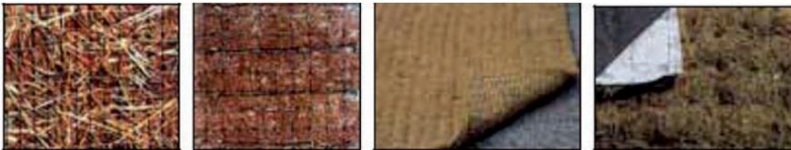
Figure 6.11: Different types of fibre mats available (www.erosionblankets.com)
