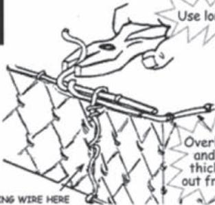
Overlap the corners and join with the thick wire sticking out from the corners.
