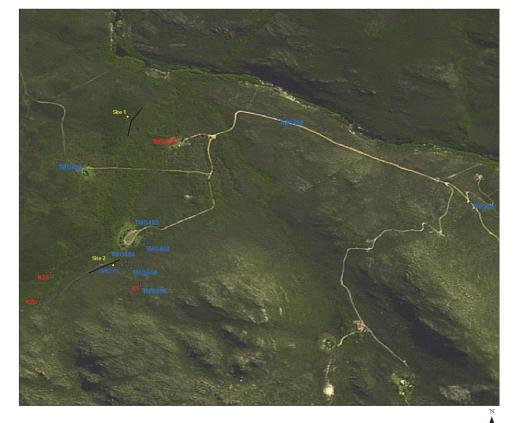
QuickBird view of the Oudebosch catchment in the Kogelberg Biosphere Reserve and monitoring points. Blue: Groundwater boreholes; Red: Piezometers and weather station (TMG538); Yellow: Soil water sensors; Black: Resistivity measurement transects.
