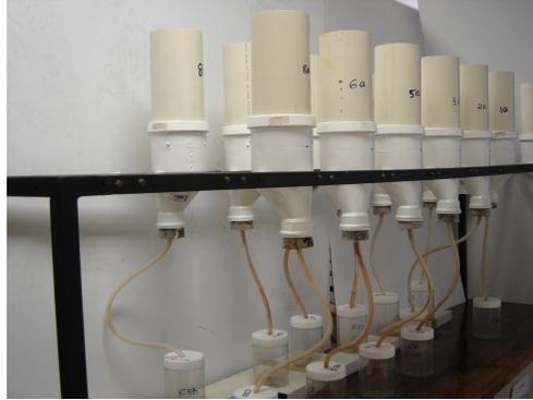
Figure 6.5: Column assembly used for the leaching experiments
