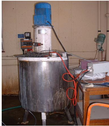
**Figure 6.4: The 150 litre capacity agitator used to generate the SR used for the drainage experiments**
