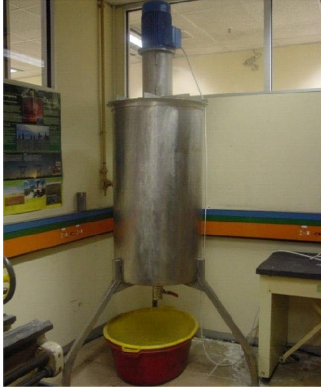
**Figure 6.76: Pilot-scale reactor used for the neutralisation of AMD with FA and preparation of SR.**
