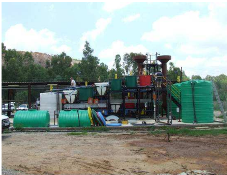
Photo 1. Pilot-plant that was used for the evaluation of the CSIR ABC Desalination Process.
