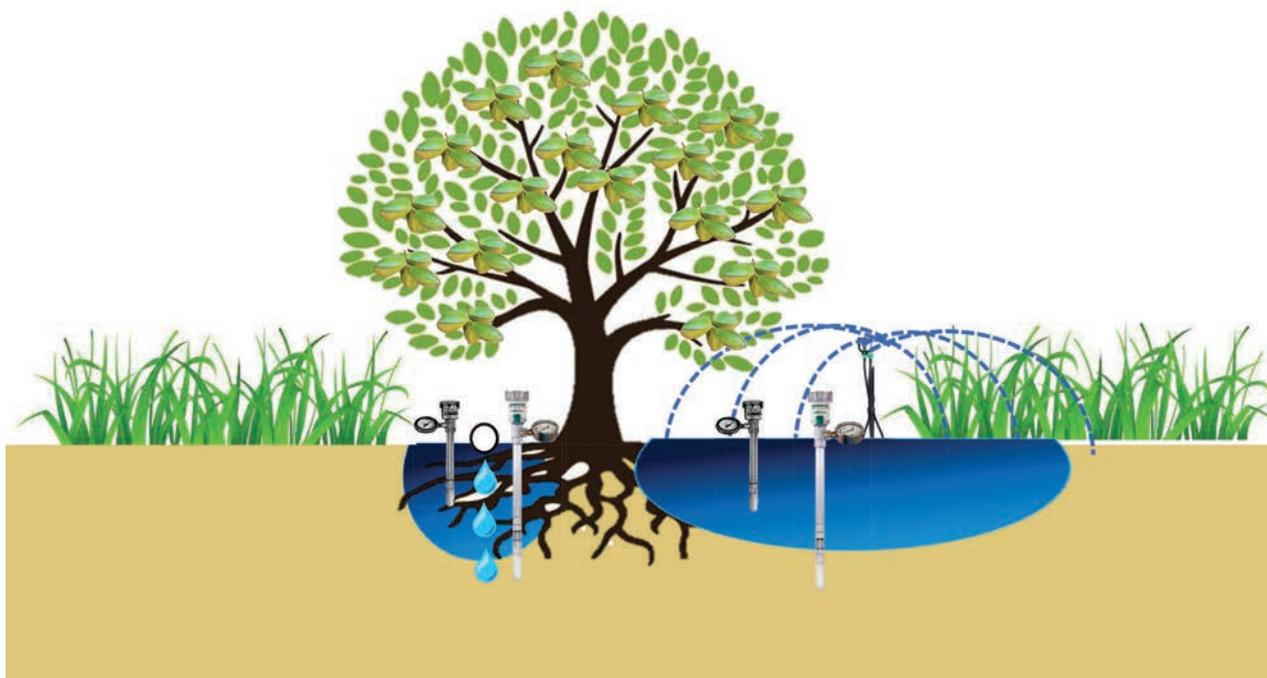
*Figure 25. Placement of tensiometers within and below the root zone to trigger irrigation events and to monitor the depth of irrigation. The shallow tensiometer indicates when irrigation should start and the deep indicates when irrigation should stop.*
