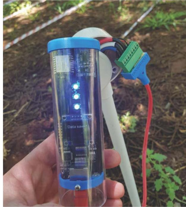
*Figure 26 Chameleon soil water sensors and wifi reader for determining soil matric potential at three different depths.*
