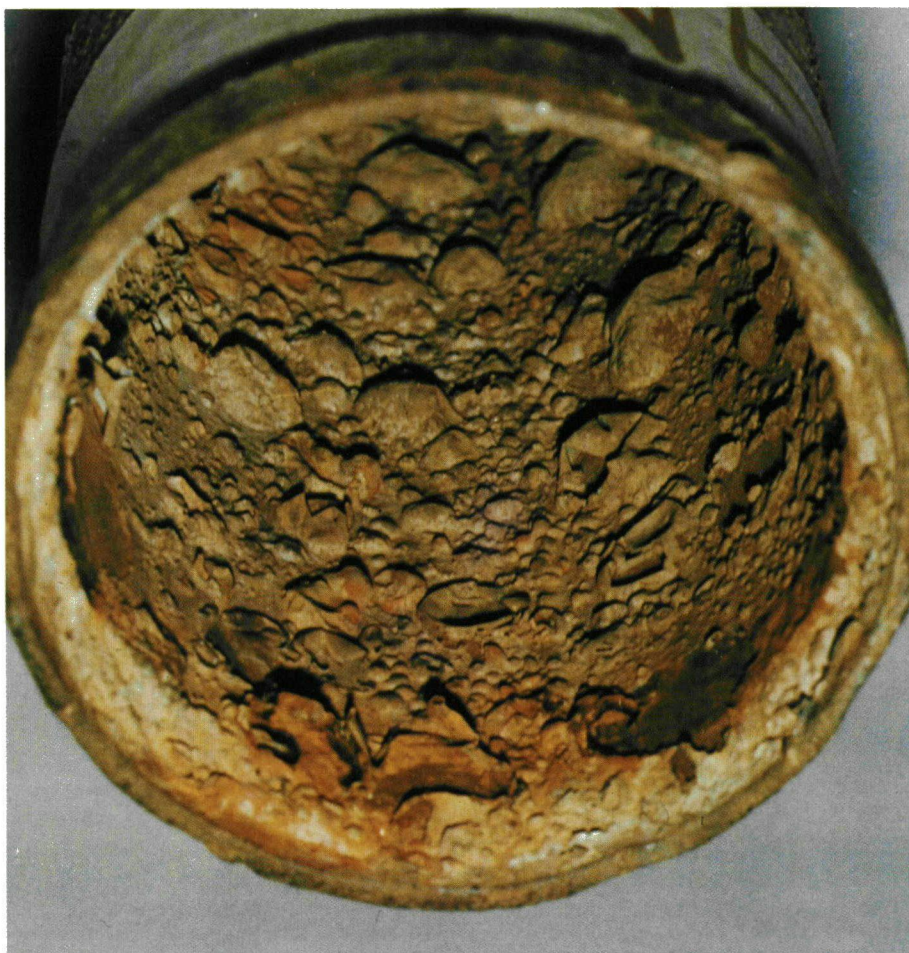
Pipe corrosion from mine service water.
