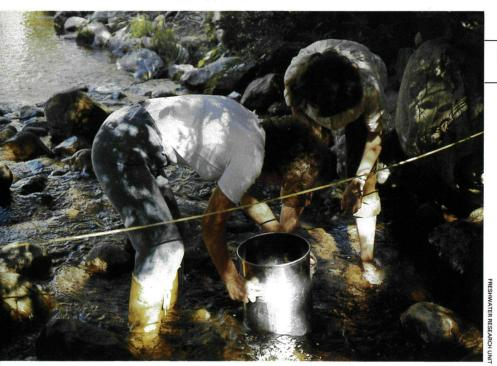
Bottom-coring in Langrivier. This technique was developed to measure accumulations of organic matter within the stream bed.
