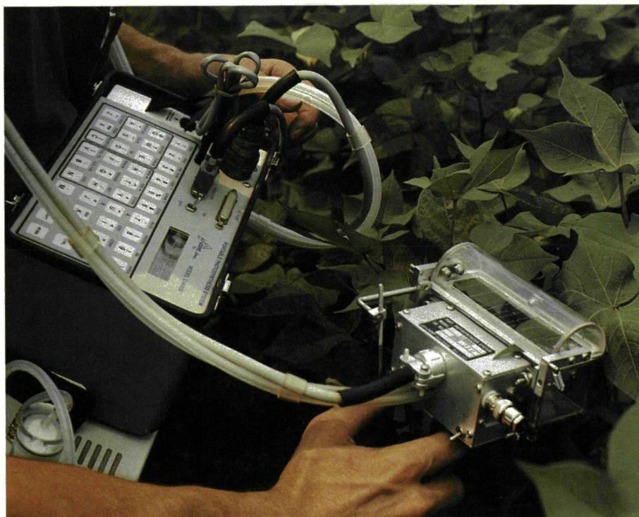
Portable photosynthesis apparatus to measure cotton leaf CO 2 uptake and stomatal resistance as an indication of plant productivity in irrigation studies.
