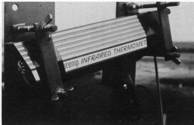
(Right) Plate 15: The infra-red thermometer gives a measure of canopy temperature and is being evaluated in irrigation scheduling studies by Mr Berliner and Dr Oosterhuis.
