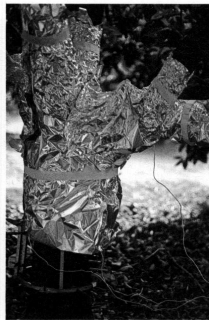
Plate 10: Thermal insulation of psychrometers inserted in the main trunk and lower branches of a citrus tree for water potential measurement. Variations in trunk diameter are recorded with the LVDT as shown.
