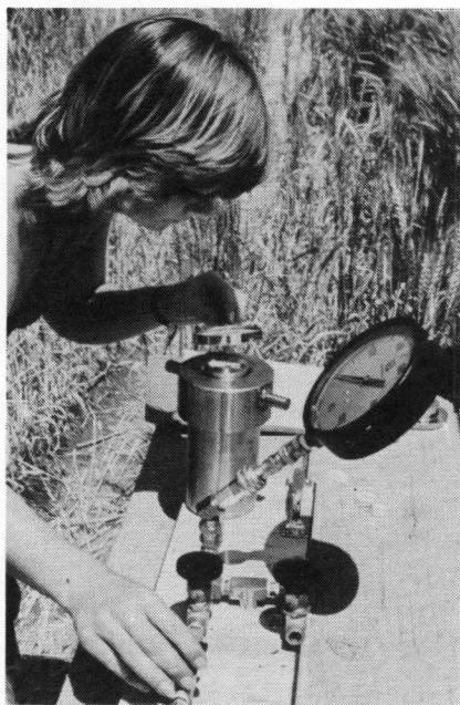
Plate 8: The pressure chamber is the most popular instrument for measuring leaf water potential. Miss Judy Eastham, operating the pressure chamber, is a soil scientist currently working on the response of leaf elongation to water stress, and also studying the importance of soil hydraulic conductivity in modelling.
