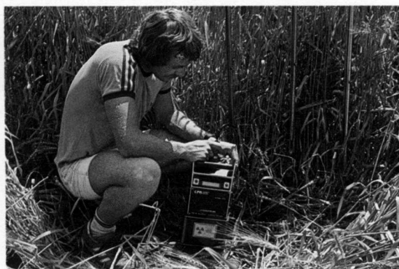
(Left) Plate 12: The neutron probe provides a measurement of soil water content at different depths in the profile. Mr Tony Proffitt has been checking calibration procedures for the neutron meter and is currently investigating root growth and plant available water.
