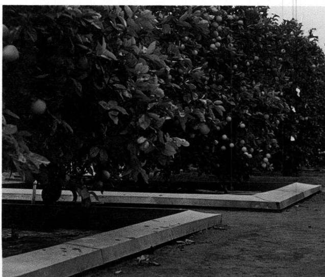
Plate 3: The lysimeters (left) provide a measure of evapotranspiration and play an integral part in the crop water use studies. The lysimeters on the left are located in a citrus orchard at Addo in the Eastern Cape and contain well established orange trees, whereas the lysimeter (right) is used for annual row crops such as soybeans.
