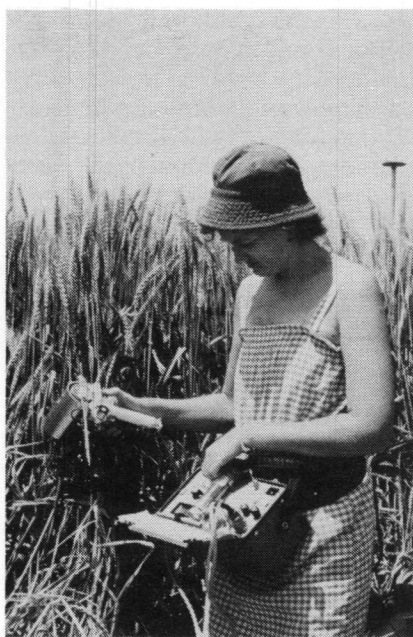
Plate 9: The steady state porometer provides a new and reliable measurement of leaf stomatal aperture. Miss Sue Walker, an agrometeorologist/plant physiologist is particularly interested in psychrometry and is involved in all measurements of plant water status including the changes that occur after the relief of stress by irrigation.
