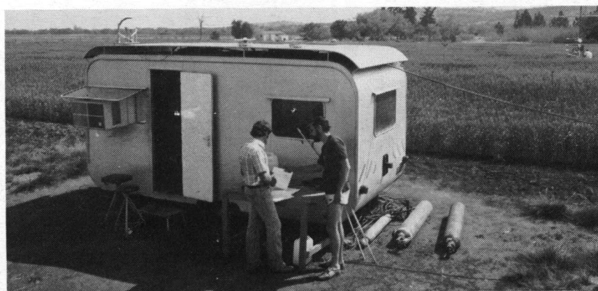
Plate 5: The caravan situated alongside the field provides shelter for the data acquisition system as well as other instrumentation used in the field studies. Dr. Derrick Oosterhuis and Mr Pedro Berliner can be seen discussing data in front of the caravan, and Mr Leon Peense, the control technician, is visible working in the field next to the instrument tower.
