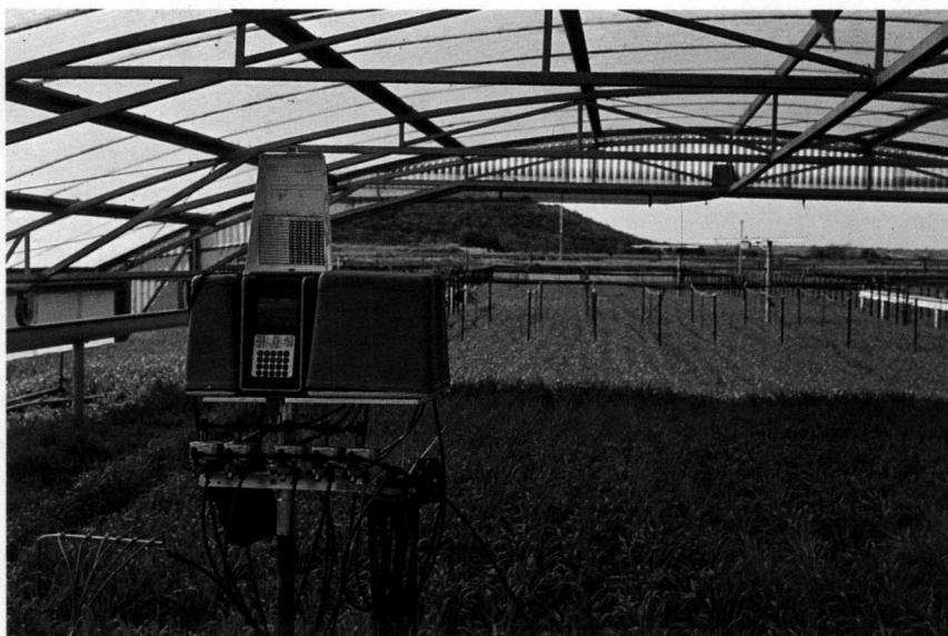
Research into crop water use and irrigation requirements at Roodeplaat. The control board for an automatic irrigation system can be seen in the foreground, as well as the rain-out shelter used to cover the plots for water stress studies.
