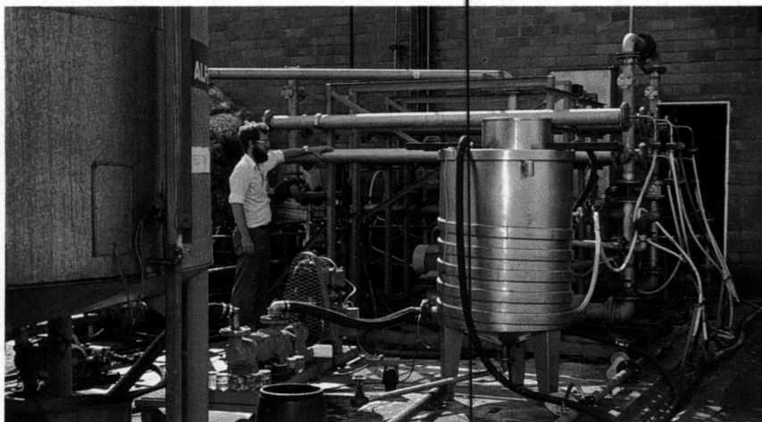
The ultrafiltration pilot plant for the treatment of sizing/desizing effluent at Messrs D Whitehead Ltd at Tongaat in Natal.
