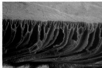
A conventional ultrafiltration membrane used for size recovery.
