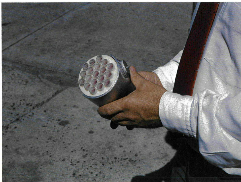
A closer view of a module showing the arrangement of the membranes.
