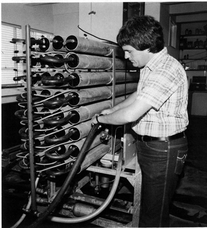
Mr Allan Hon of National Institute for Water Research in Bellville pictured with the Bakke reverse osmosis pilot plant used in the research project.
