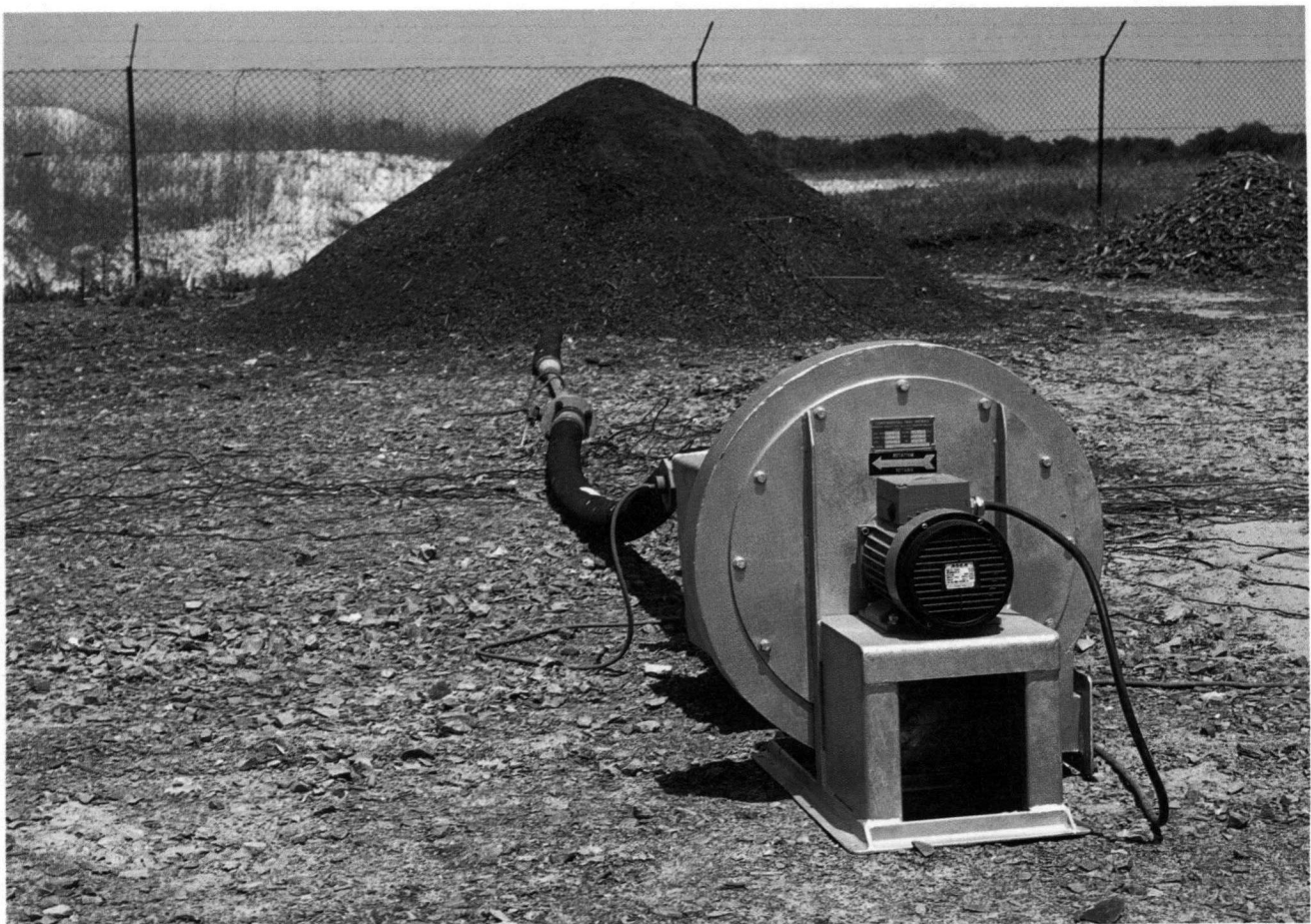
A pile of sludge mixed with woodchips undergoing biothermal stabilisation during which temperatures in excess of 70°C are readily achieved. The aeration fan is seen in the foreground.
