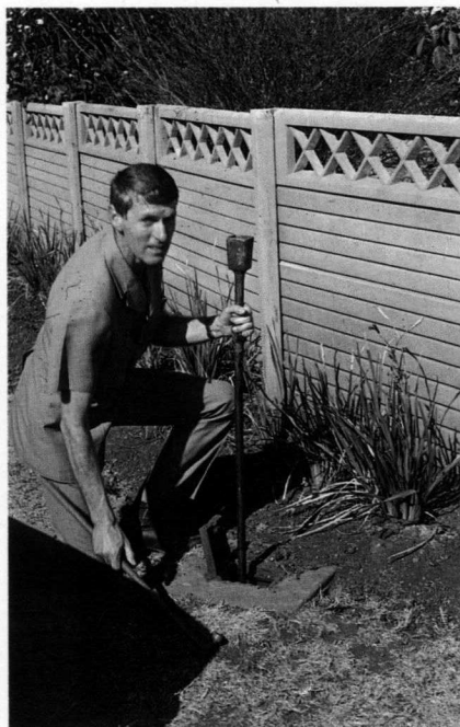
George Malan, NBRI, preparing to close and isolate valves prior to the step testing.
