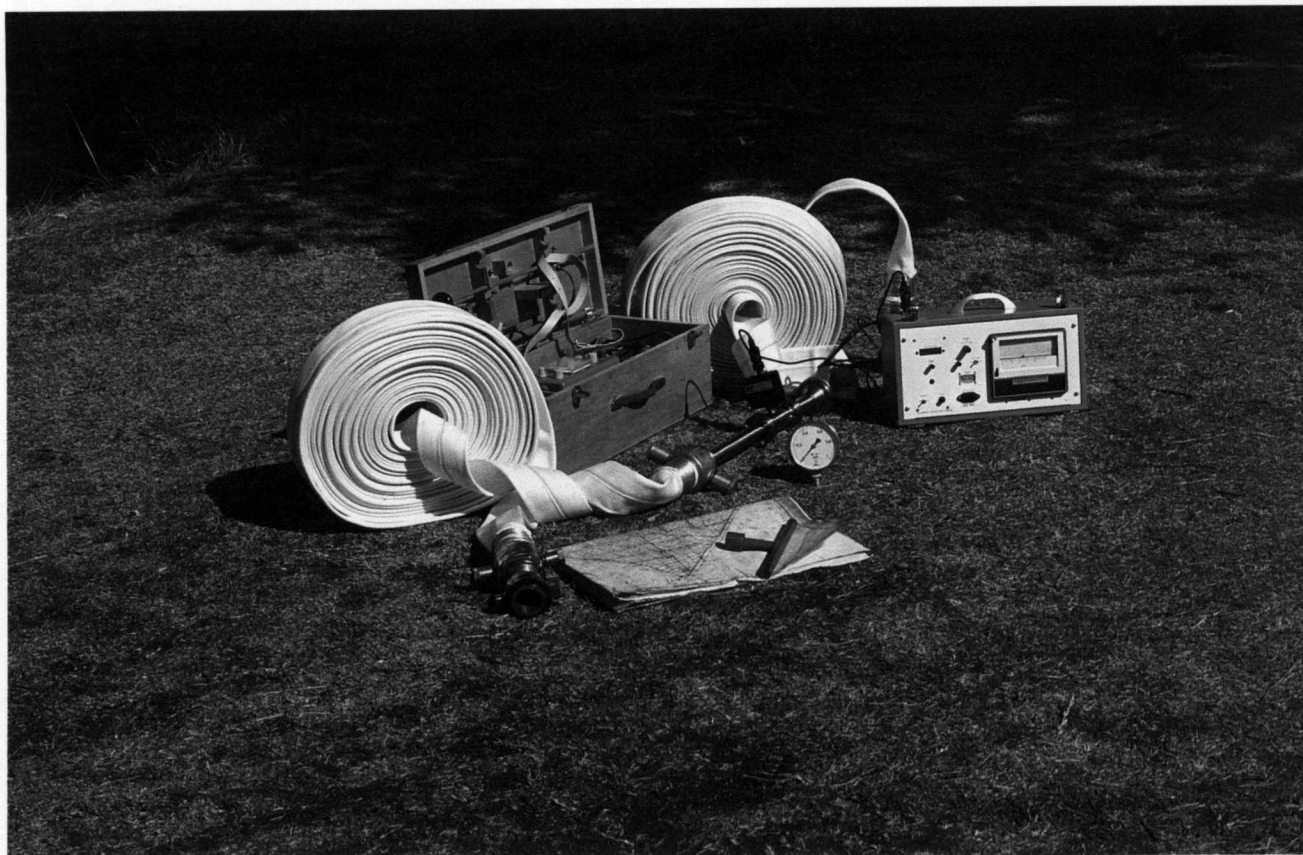
Illustrated above is the equipment for establishing that a leak exists. In front of the wooden box containing sounding equipment, is the special waste water meter with its electronic flow recorder and fire hoses used to bypass the isolating valve.
